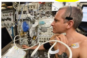
ESA ECHO hardware uses both Remote Guidance Ultrasound (voice) with simultaneous operation of Robotic Motorized Probes (Photo credit: D. Chaput)
