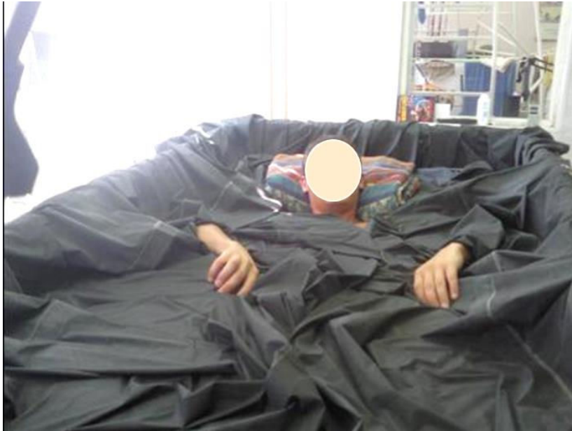
Fig. 4.1: Photograph of a participant submerged in the DI tank. Waterproof bags are used to contain the water and to provide a dry environment for the participant.
