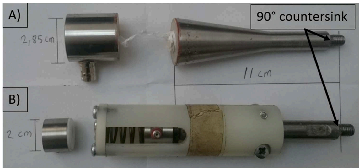
Figure 17. Two options for the waveguide setup. A) The failed LNWDI sensor and B) the one used in most tests, with a regular size sensor fixed inside the waveguide, and another similar sensor outside the casing.
