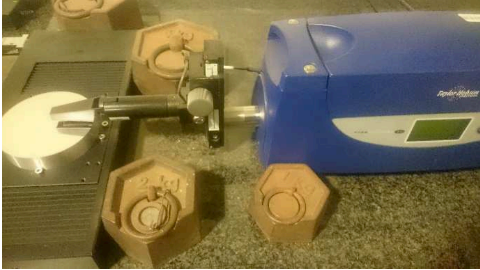
Figure 18. The contact profilometer measuring a specimen profile. The stainless steel specimen is in the left and the profilometer measures the radial profile.
