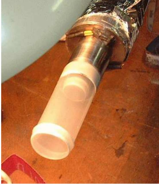
FIGURE (2.2) LH<sub>2</sub> target used to study elementary processes [104].
