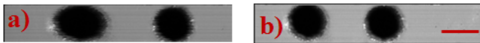
Figure A.7: Comparison of scan images of circular holes in a LiNbO 3 crystal (fast direction is the horizontal). (a) With a trapezoidal scan and theoretical values of offset. (b) With a corrected scan. Scale-bar 40\mu\text{m} .
