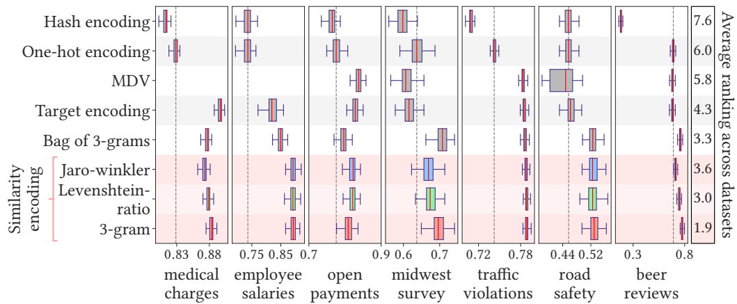
Figure 7.1 – Performance of different encoding methods. Classifier: gradient boosting. Each box-plot summarizes the prediction scores of 100 random splits (with 80% of the samples for training and 20% for testing). For all datasets, the prediction score is upper bounded by 1 (a higher score means a better prediction). The right side of the figure indicates the average ranking across datasets for each method. The vertical dashed line indicates the median value of the one-hot encoding method. Similar results are obtained for a linear classifier (see Figure C.1 in the Appendix).
