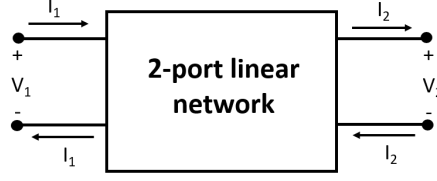
Fig. 2.14 2-port linear network representation
