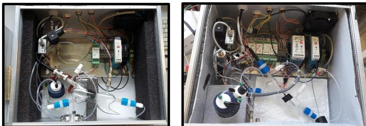
**Figure 2.14:** LSCE-CRM new set-up. On the left the first version with a stainless-steel 4-way valve for switching between dry and wet N<sub>2</sub>, with no heating of the line between the water reservoir and the reactor. On the right, the second version with a Teflon 4-way valve and a heated/covered line conducting nitrogen to the reactor, with several temperature sensors.
