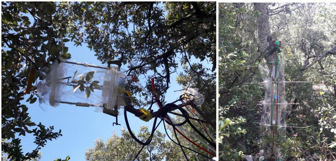
**Figure 5.1:** Photos of the branch (left) and stem chambers (right) used during the COV<sup>3</sup>ER- 2018 Puéchabon field experiment.
