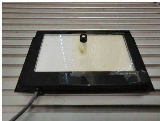
*Figure 0-1: LED panel used for photocatalytic experiment*
