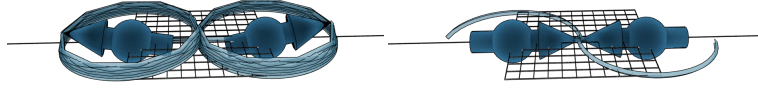
Figure 2.6: A small canting triggers precession around the net magnetization axis. Left: initial canting of 25^\circ with its induced precession. Right: initial canting of 1.5^\circ resulting in an orientation swap.
