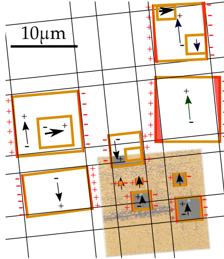
Figure 3.24: Explanation of the ferroelectric orientation. The orientation of \mathbf{P}_e is caused by a charge accumulations at the edges of the pattern due to the missalignment of the squares with respect to the diagonals of the crystal axis (black lines).
