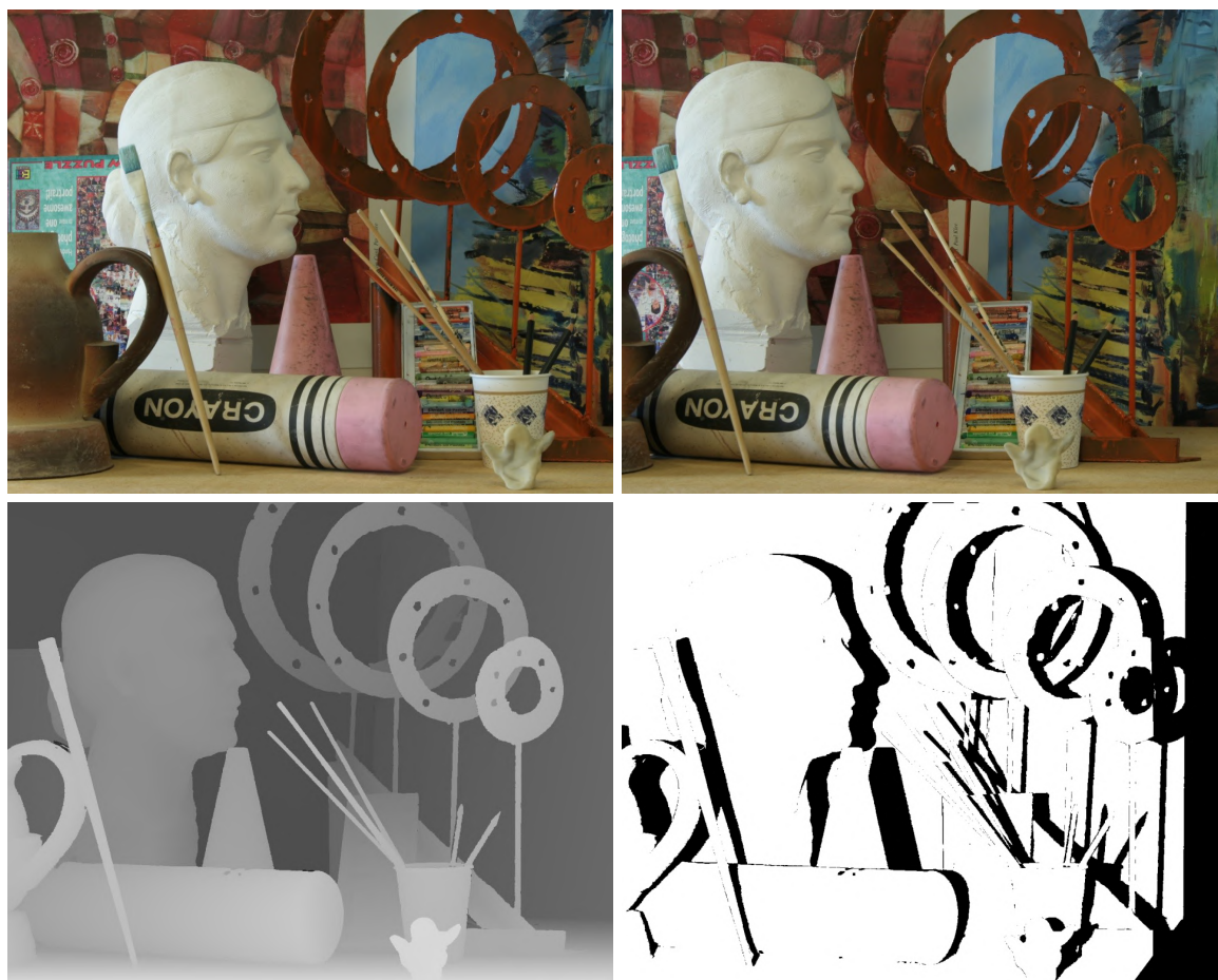
Figure 7.14 – "Art" stereo pair. From left to right: left and right views (top), disparity map with holes filling of the right view and occlusion map of the right view. Occluded regions appear in black.
