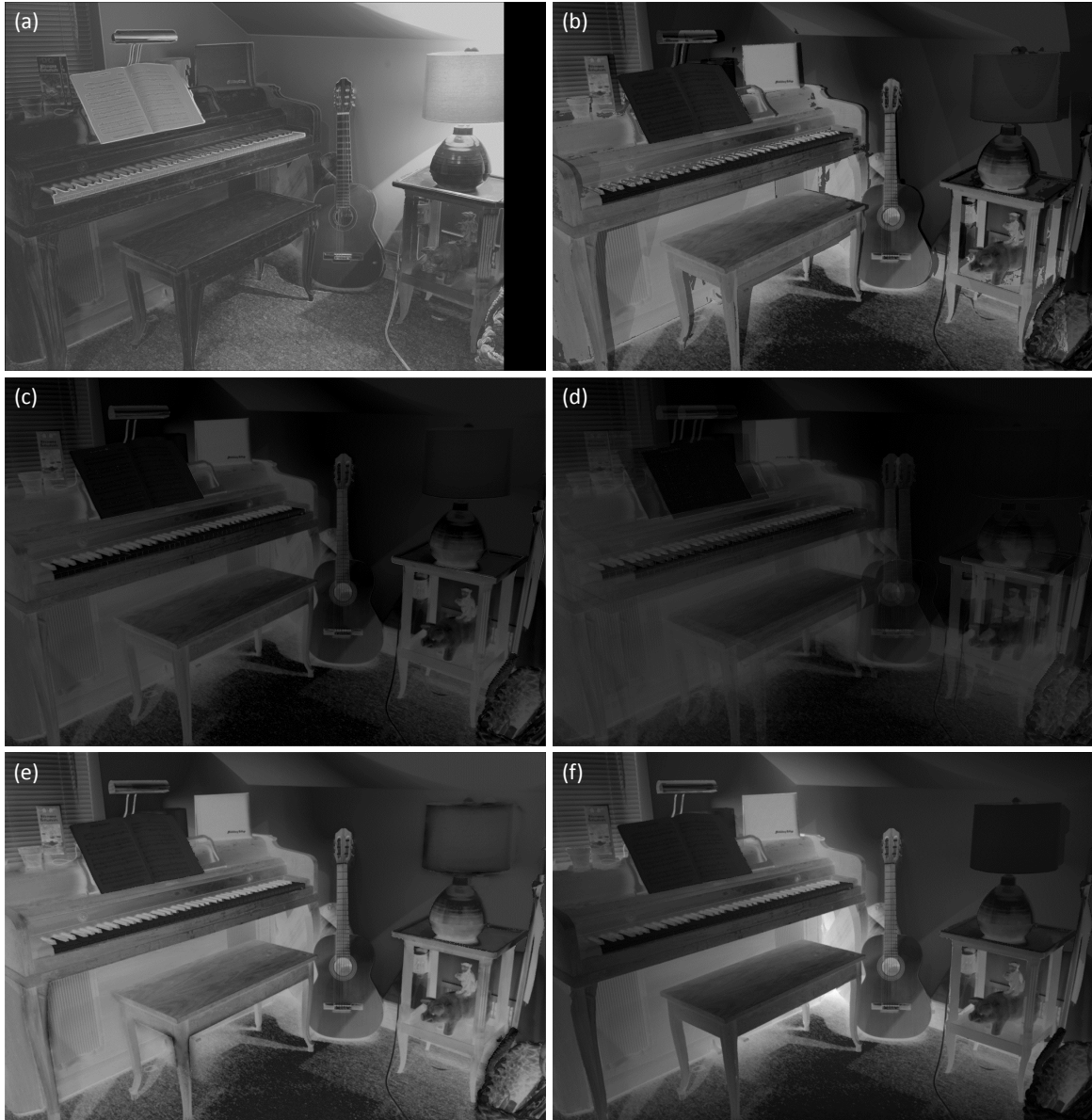
Figure 7.19 – JND profiles of "Piano" stereo pair obtained using different 3D-JND models. (a) BJND map, (b) JJND map, (c) MJND map, (d) SJND map, (e) HJND map, (f) DJND map.
