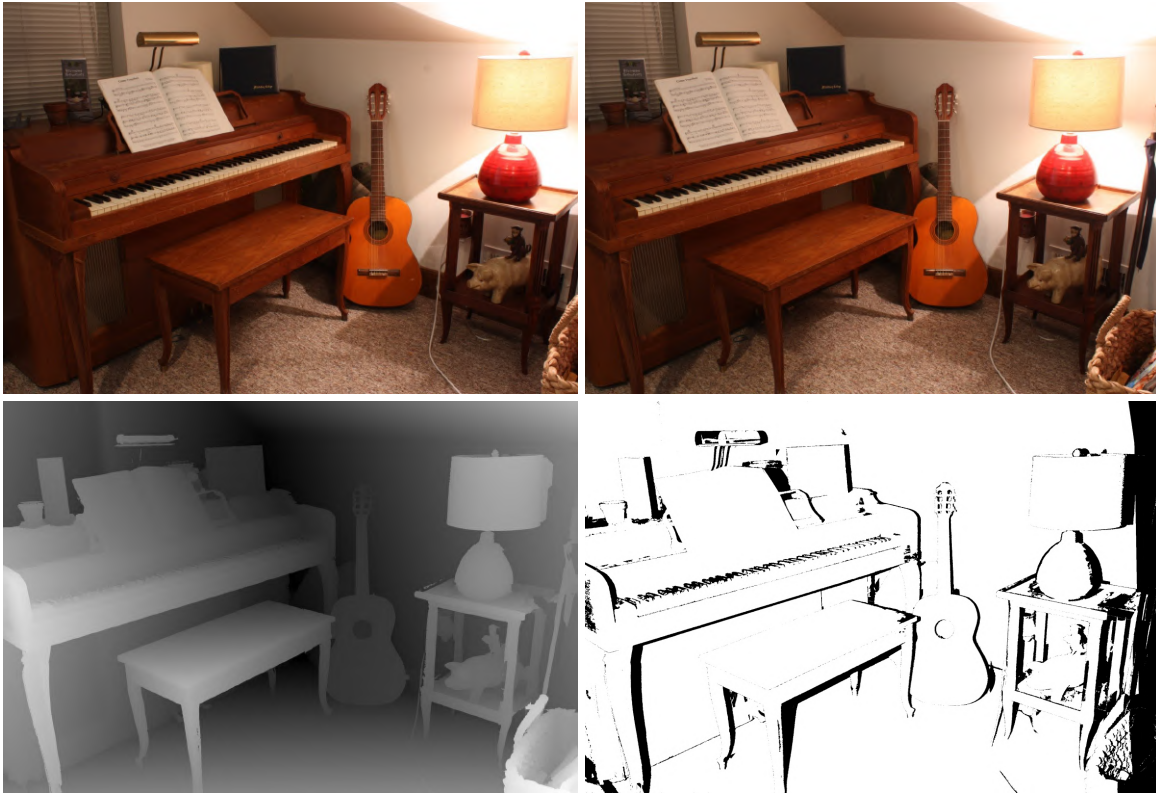
Figure 7.18 – "Piano" stereo pair. From left to right: left and right views (top), disparity map with holes filling of the right view and occlusion map of the right view. Occluded regions appear in black.
