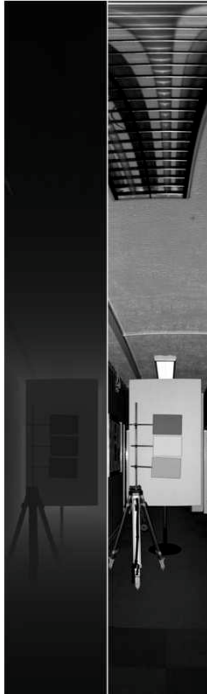
Figure 4.8 – Equirectangular Range image (left) and intensity image (right). Values displayed as grayscale, lowest black, highest white.
