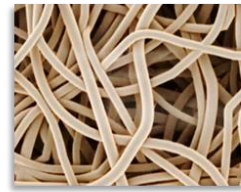
Cellulose nanofibrils Length several \mu\text{m} Width 5-50 nm
