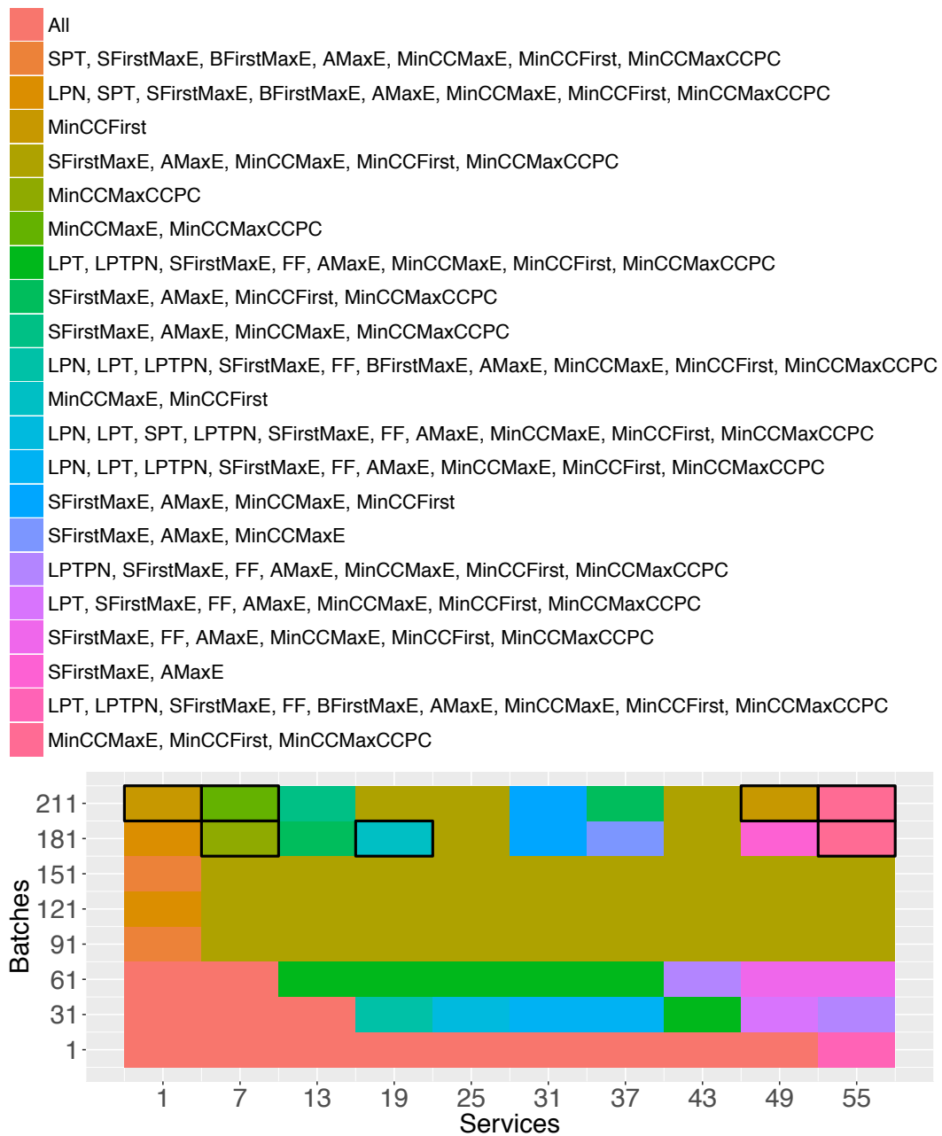
Figure 5.26: Highest total profit comparison with cross-correlation algorithm with power profile 1 for all workload variations.
