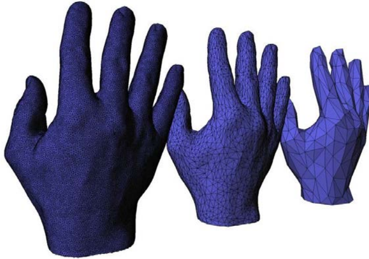
Figure 2: Triangular mesh decimation [Cac19]. The complexity of the topology describing the geometry of the mesh is reduced.
