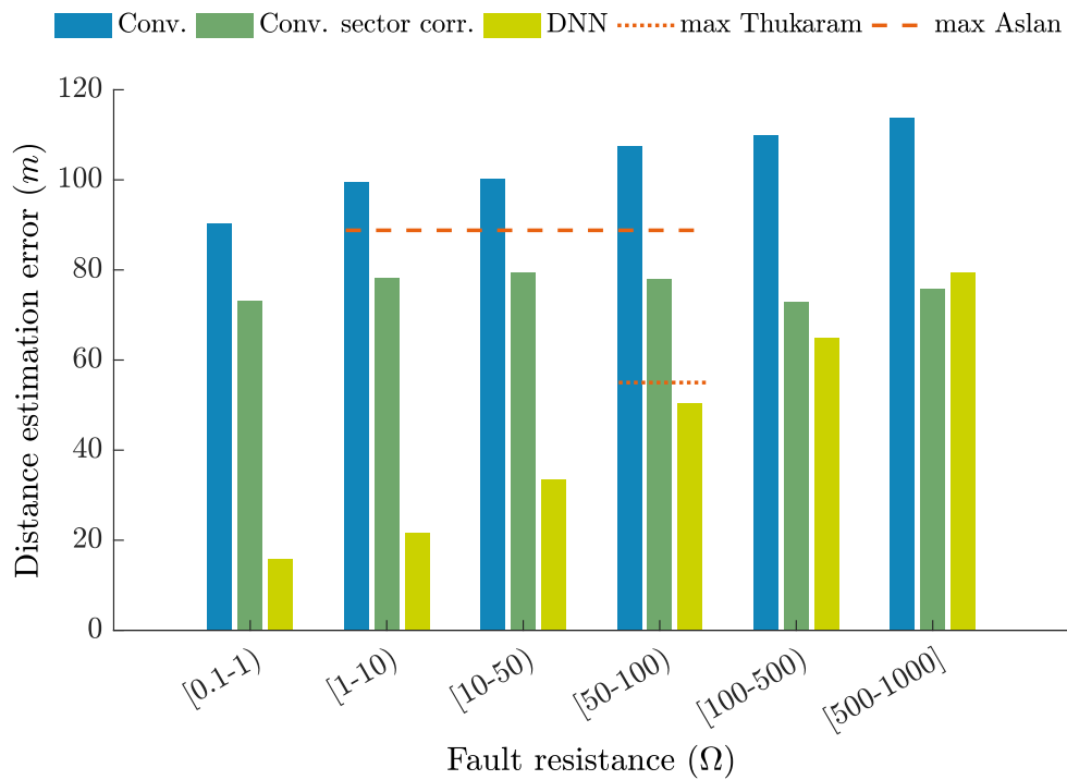
Figure 6.3 Fault distance estimation error in meters per fault resistance values for the two developed methods compared to two from the literature.
