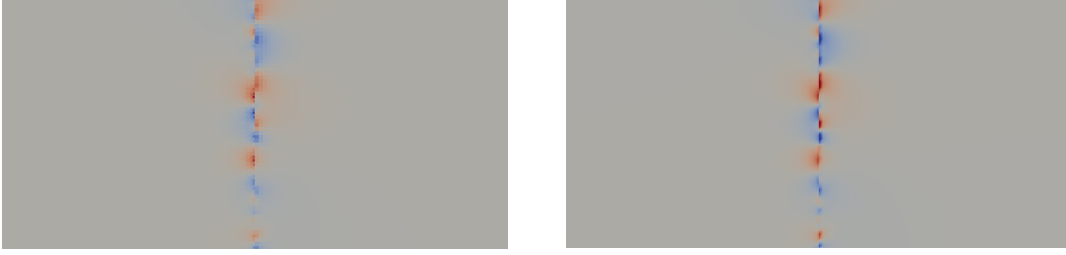
Fig. IV.8 Error \mathbf{u}_{\mathcal{T}}^0 - \mathbf{u}_{\mathcal{T}} at the 10^{th} iteration. Left: Primal mesh, \|\mathbf{u}_{\mathcal{M}}^2 - \mathbf{u}_{\mathcal{M}}\|_{\infty} = 0.52 . Right: Dual mesh, \|\mathbf{u}_{\mathcal{M}^* \cup \partial \mathcal{M}^*}^2 - \mathbf{u}_{\mathcal{M}^* \cup \partial \mathcal{M}^*}\|_{\infty} = 0.05 .
