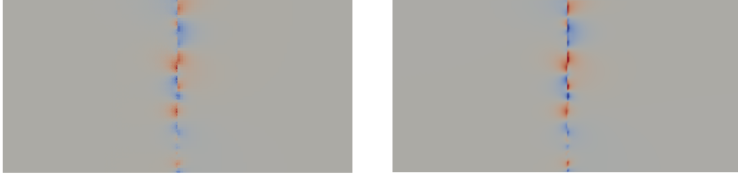
Fig. IV.8 Error \mathbf{u}_{\mathfrak{T}}^0 - \mathbf{u}_{\mathfrak{T}} at the 10^{th} iteration. Left: Primal mesh, \|\mathbf{u}_{\mathfrak{M}}^2 - \mathbf{u}_{\mathfrak{M}}\|_{\infty} = 0.52 . Right: Dual mesh, \|\mathbf{u}_{\mathfrak{M}^* \cup \partial \mathfrak{M}^*}^2 - \mathbf{u}_{\mathfrak{M}^* \cup \partial \mathfrak{M}^*}\|_{\infty} = 0.05 .
