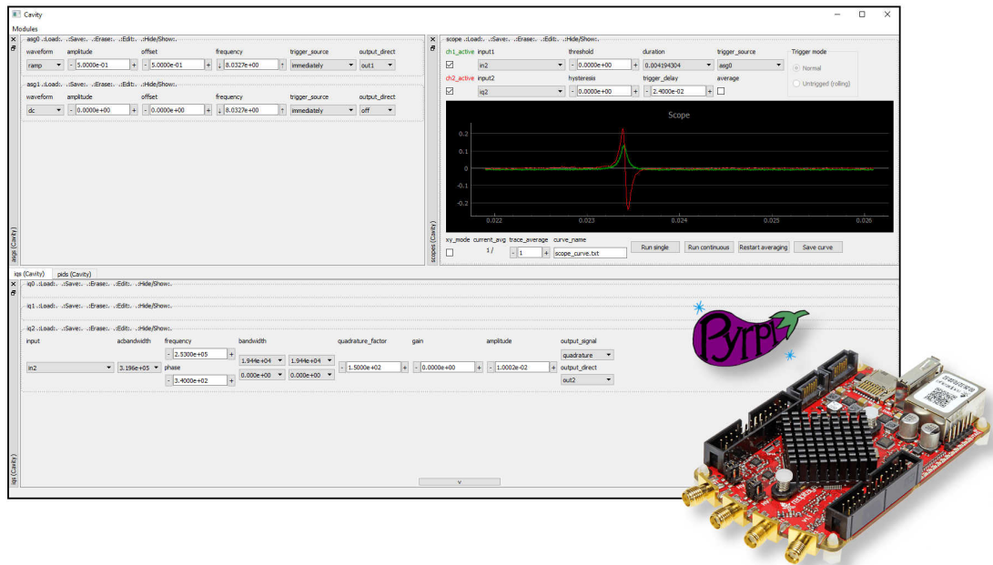
FIGURE 5.3 – Interface of the PyRPL software used to control the Red-Pitaya FPGA card (inset).
