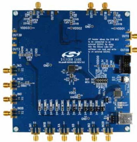
Figure 49. External PLL development board. SI5342 Silicon Labs. (Photo: from datasheet)
