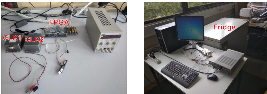
Figure 53. Test Bench. The gray boxes contain a clock and a temperature sensor. The white box in the background is the fridge.
