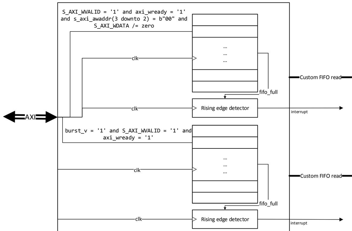
**Figure 3.16** – Simplified schematic of the optimized instrumentation IP.
