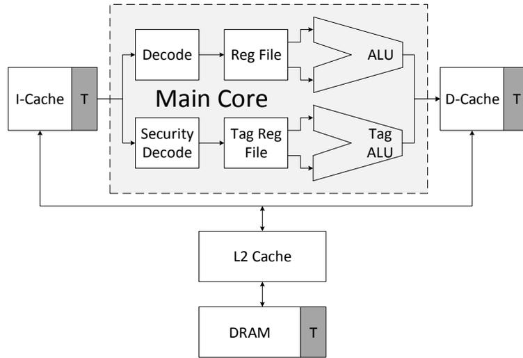
Figure 2.4 – In-core DIFT (adapted from [2]).
