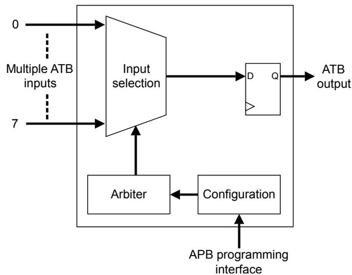
Figure 3.5 – CS Funnel (Link class component).
