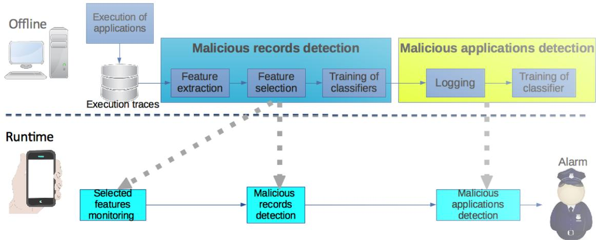
Figure 6.1 – Proposed detection system (taken from [16])
