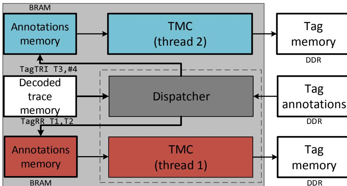
Figure 5.12 – DIFT coprocessor for multiple threads.
