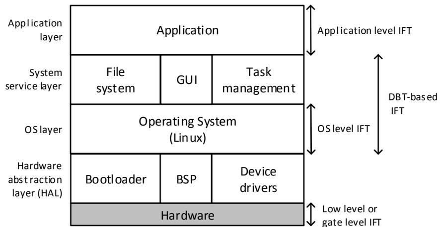
Figure 2.2 – Software architecture of an embedded system.
