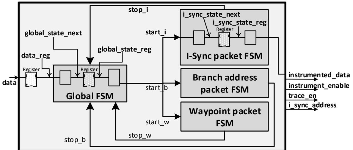
Figure 3.9 – Overall architecture of PFT Decoder.
