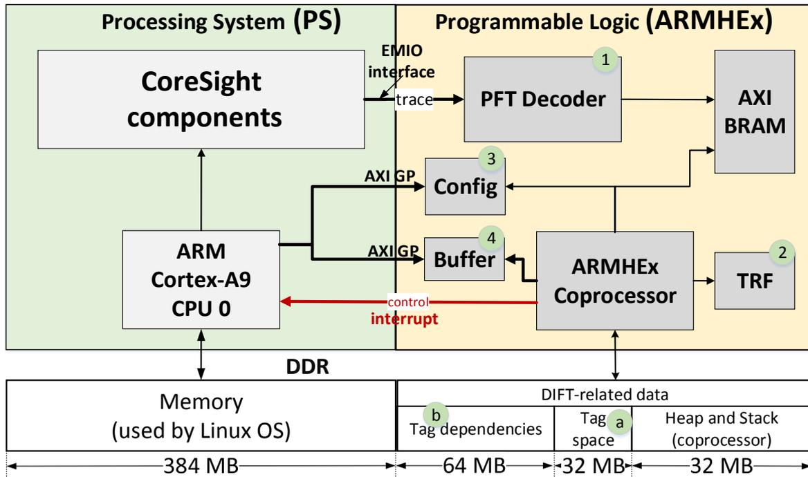
Figure 4.2 – Internal architecture of an ARMHEX-based system.
