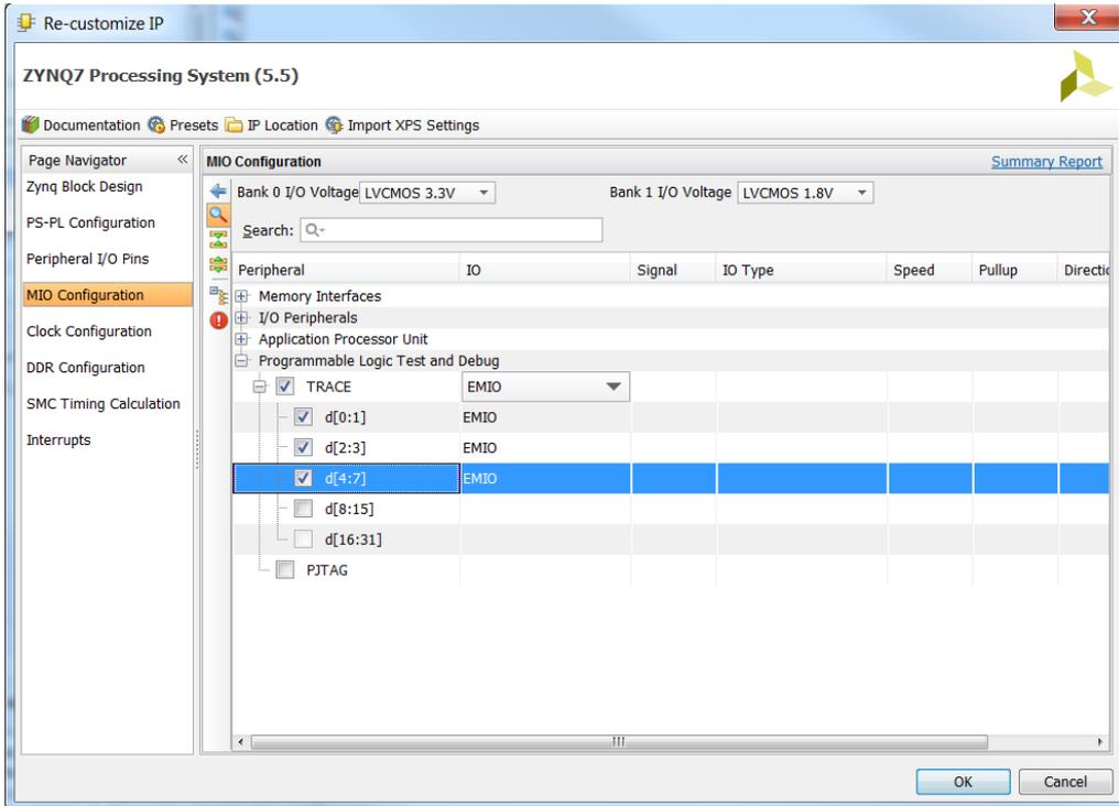
Figure 3.7 – TPIU trace connected to EMIO using Xilinx Vivado.
