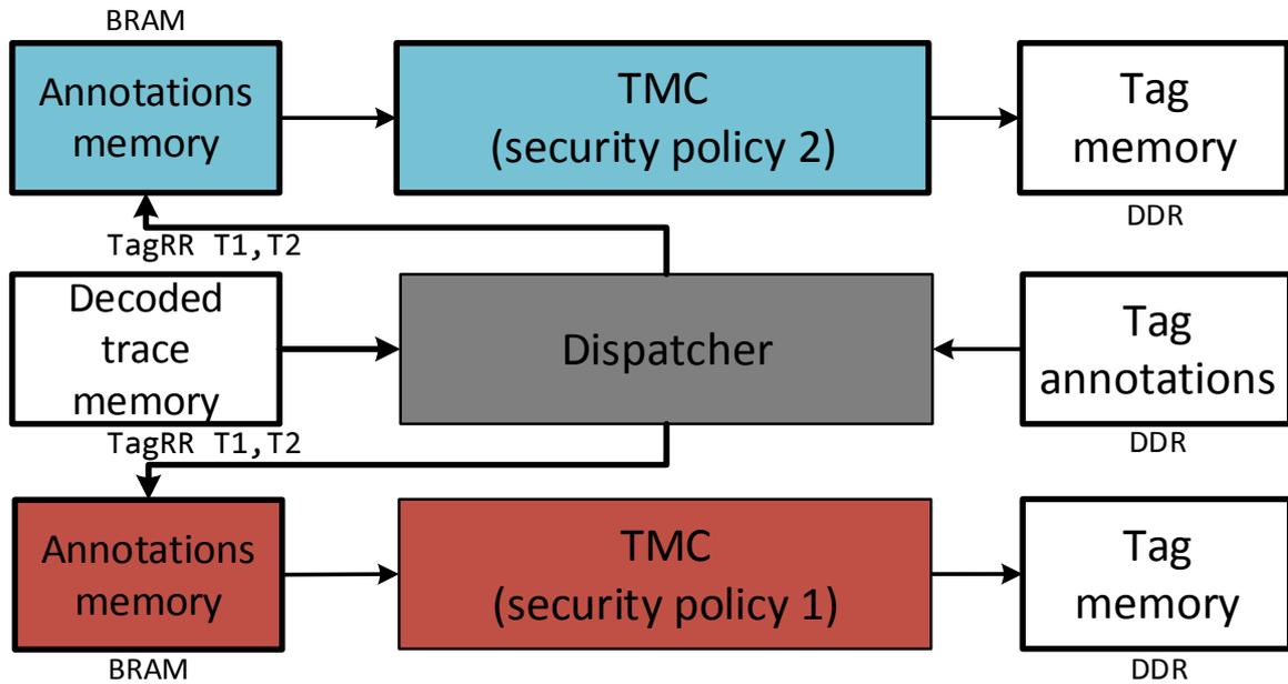
Figure 5.11 – DIFT coprocessor for multiple security policies.
