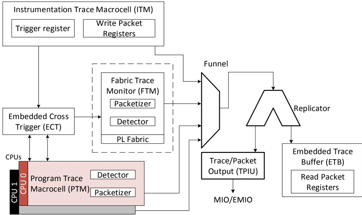
Figure 3.2 – CS components in Xilinx Zynq [55].
