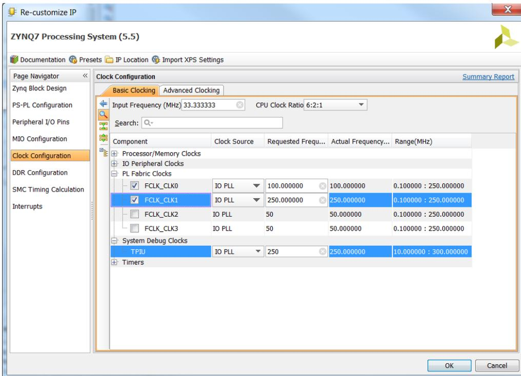
Figure 3.8 – TPIU trace clock configuration using Xilinx Vivado.
