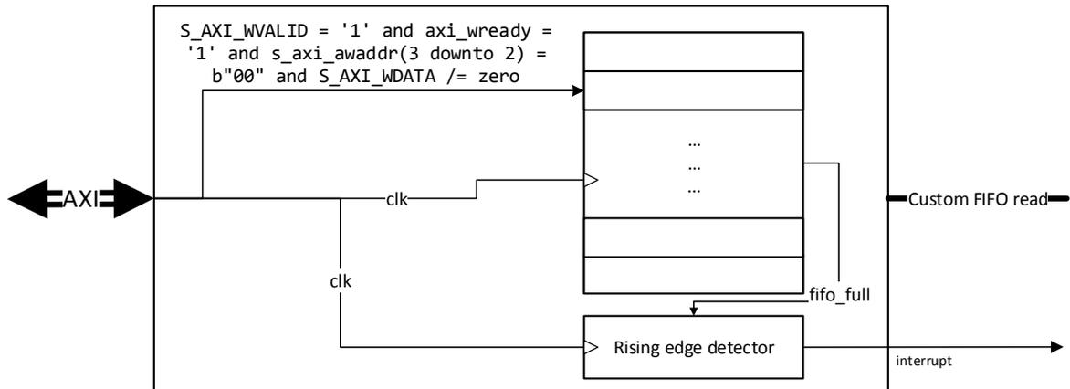
**Figure 3.15** – Simplified schematic of the instrumentation IP.
