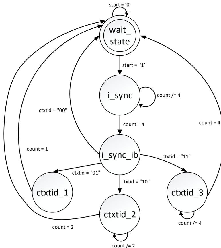
**Figure 3.10** – State machine diagram for I-sync packet.
