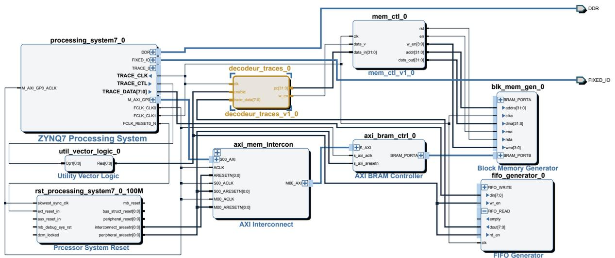
**Figure 3.13** – This design shows how to use PFT Decoder. Trace is sent to the `decodeur_trace` IP which takes care of decoding trace packet in order to obtain control flow addresses of the program that is being executed on the ARM core. The decoded trace is stored in `blk_mem_gen_0` IP to read it back from the ARM core using the second port of the BRAM.
