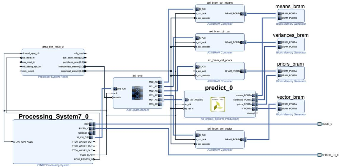
**Figure 6.3** – This Figure shows the Vivado design used in order to verify the hardware version of the NB algorithm (**predict\_0** IP). The Zynq **Processing\_System7\_0** IP represents the configuration of the ARM core on the Zynq SoC. The ARM core sends the data to the **predict\_0** IP and recovers the return data in order to verify it with the result of software version. The ARM core also takes care of measuring the execution time for both software and hardware versions.
