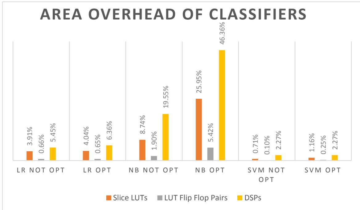
**Figure 6.5** – Area overhead of the implemented algorithms using optimized and non-optimized hardware IPs. The non-optimized versions are more area efficient while the optimized versions require more FPGA area. As the goal of the optimization is to improve both power and performance overhead, the area taken by the optimized version is higher than the non-optimized hardware version.
