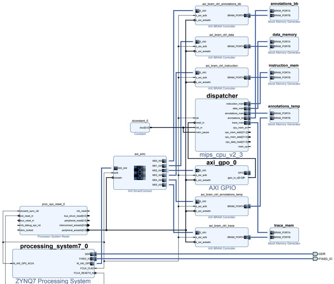
**Figure 5.8** – This Figure shows the design made in order to implement the dispatcher core on the FPGA and evaluate it on the FPGA. The Zynq **Processing\_system7\_0** IP is used in order to initialize the content of instruction memory (**instruction\_mem**)
