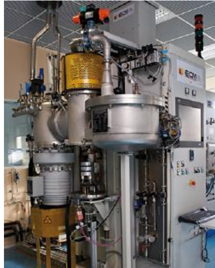
Fig. 27: Furnace used at CEA-LITEN for sintering, annealing and diffusion heat treatments.
