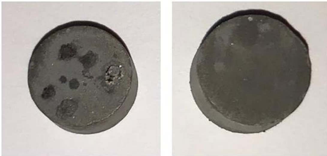
Fig. 77: (Left) Image of the surface state of a magnet diffused with the eutectic alloy Dy_{66}Co_{34} . (Right) Same for a magnet diffused with the intermetallic compound Dy_{63}Co_{37} .
