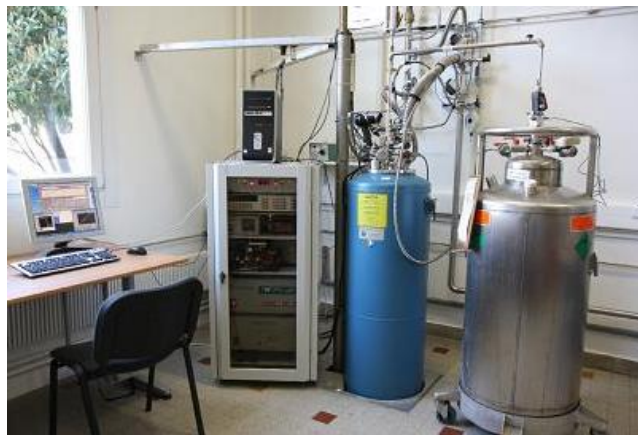
Fig. 36: Extraction magnetometer used at Institut Néel for magnetic characterization in open-circuit conditions.
