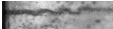
Figure 3.22: PF1 during CWM1 at SP2 (2245 Hz) - Backlighting image obtained with the APX camera. The liquid jet oscillates due to the acoustic modulation.
