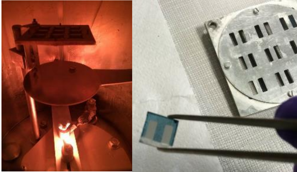
Figure 2-6: Physical vapour deposition of the Ag electrode (left) and removal of the device from the shadow mask (right), prior to removal of excess polymer.
