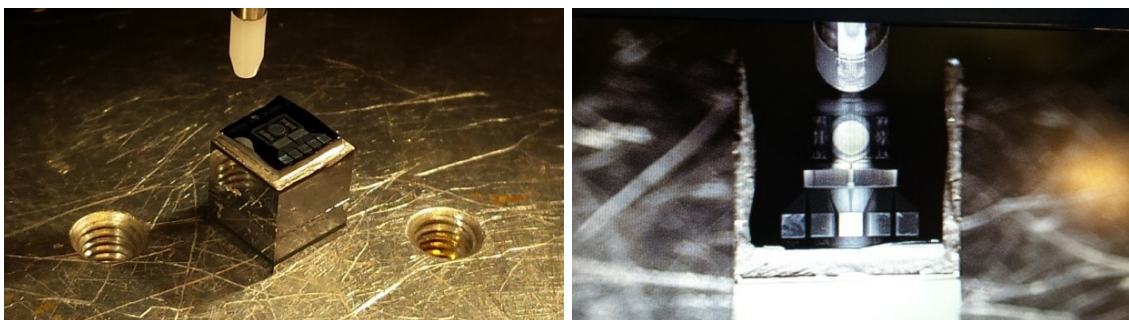
Figure 6.22: Micro-scanner bonded to the interferometer-chip.
