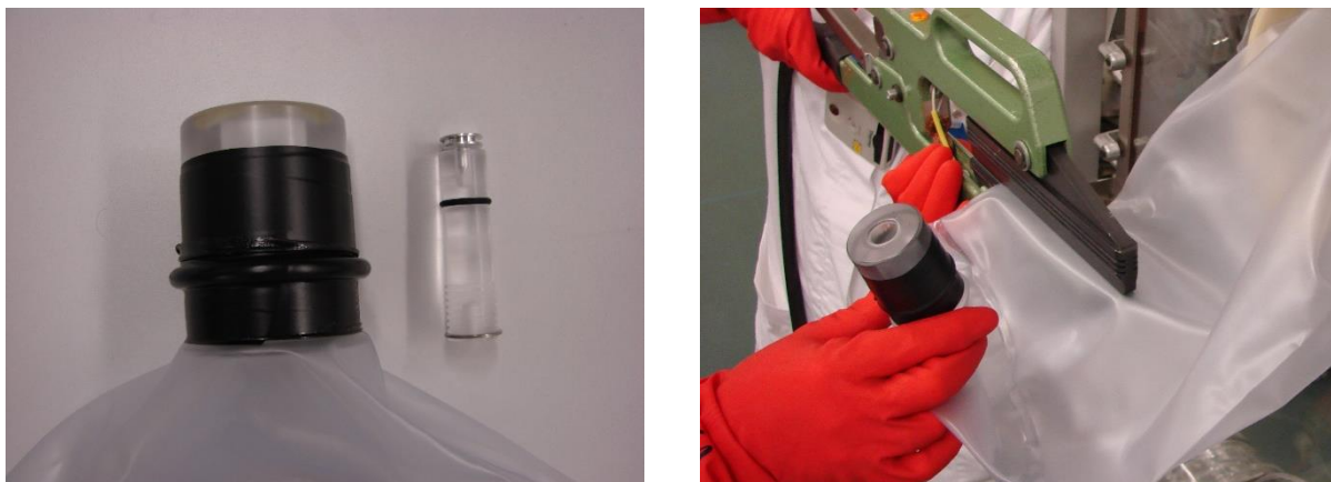
Figure 43: sample holder connected to the bag (left) and bag-out operation of a loaded sample holder from a glovebox at JRC-KA. (196)
