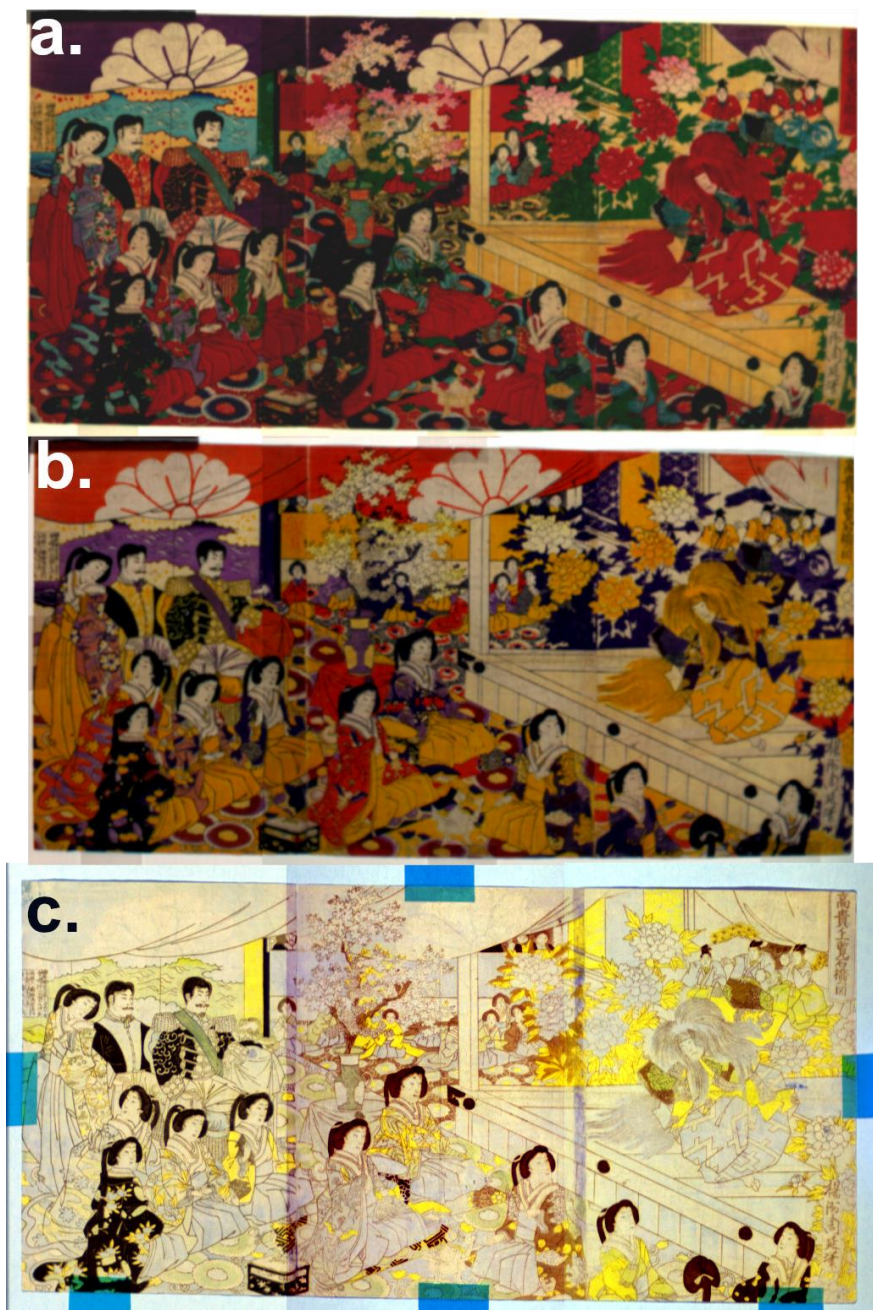
Figure IV.21. Images hyperspectrales VNIR et SWIR de l'estampe 49887_Chikanobu : a. image RGB (650, 540, 450 nm) (HSI VNIR IQ) ; b. image IRFC (900, 650, 540 nm) (HSI VNIR IQ) ; c. images SWIRFC (FC1, 4058, 5141, 9940 \text{cm}^{-1} ) (HSI SWIR)
