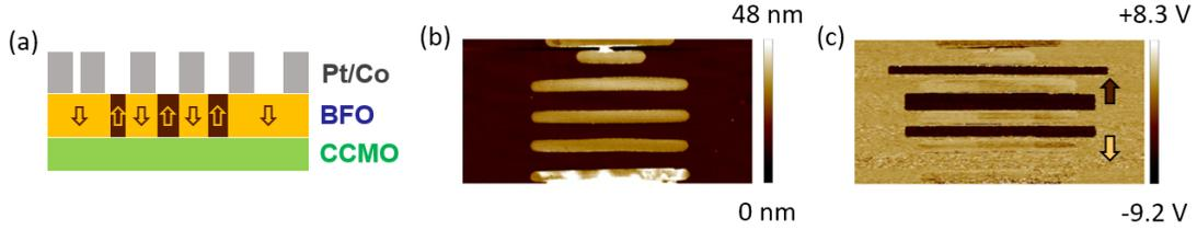
Figure 5.5: (a) Schematic of the lamella used for the STEM experiments.  $20 \times 20 \mu\text{m}^2$  images of (b) the topography and (c) the ferroelectric polarization of the bilayer with deposited metal markers before focused ion beam lithography.
