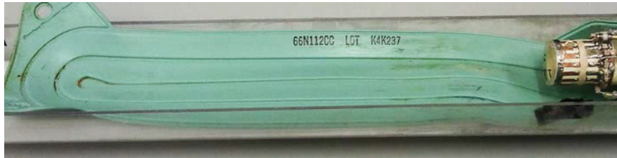
Figure II-52: Warming pad placed on the coil holder next to the coil to control mouse body temperature from underneath.
