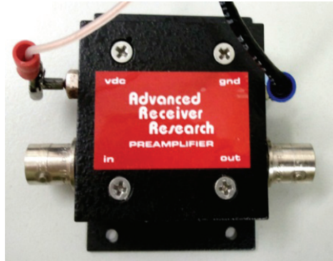
Figure III-29: Our low-noise figure pre-amp purchased from Advanced Receiver Research
