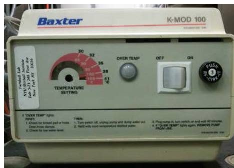
Figure II-53: Water pump with built-in heating system
