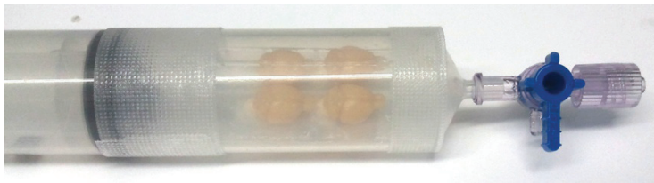
Figure III-3: The brain setup was placed inside a syringe with a stopcock lock.
