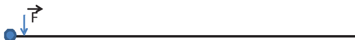
Figure I-3: Causing a vibration by applying a force at one end of the string
