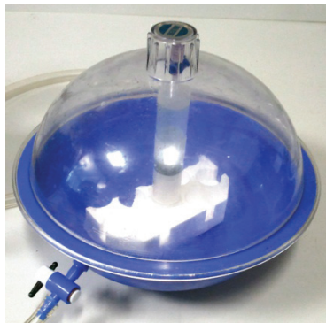
Figure III-4: Vacuum chamber for degassing.
