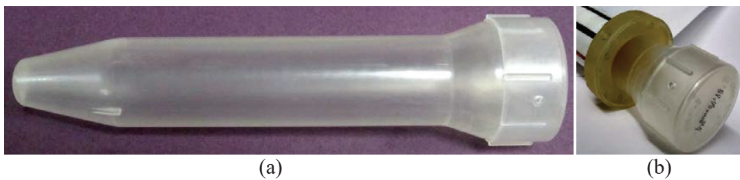
Figure II-30: a) cylindrical plastic holder to characterize the coil's homogeneity. B) Holder fits perfectly in the coil.
