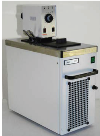
Figure II-55: Second water pump with built-in heating system to control mouse body temperature from top.
