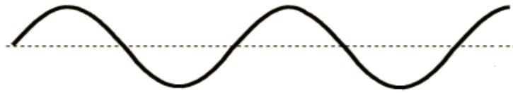
Figure I-4: Transverse wave traveling along the string
