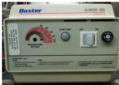
**Figure II-53:** Water pump with built-in heating system
