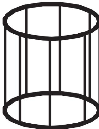
Figure II-1: *Inducting element of a birdcage coil*
