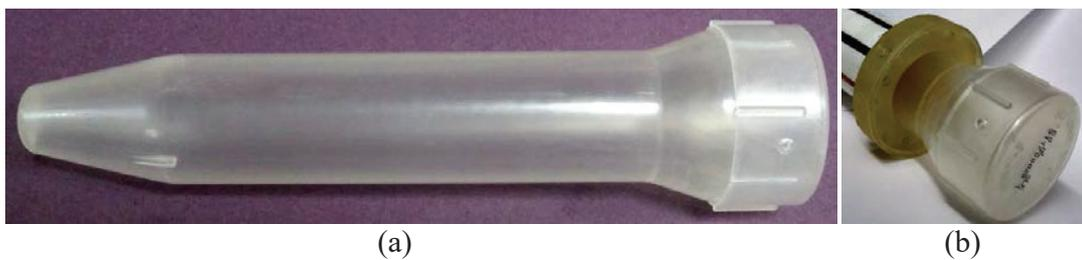
**Figure II-30:** a) cylindrical plastic holder to characterize the coil's homogeneity. B) Holder fits perfectly in the coil.
