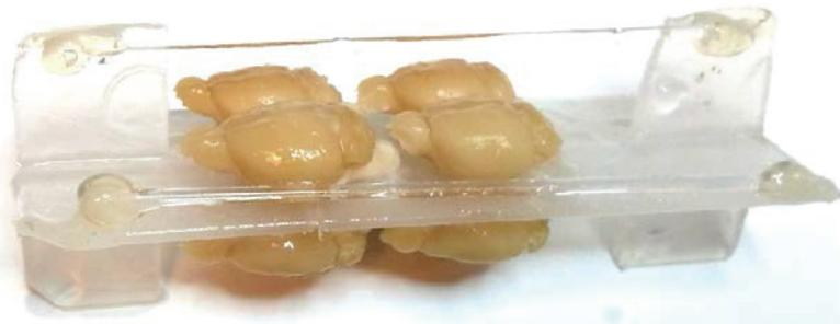
**Figure III-18:** *8-brain setup for high throughput scans*
