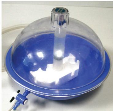
**Figure III-4:** Vacuum chamber for degassing.
