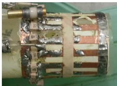
**Figure II-48:** *Homemade Litz cage*
