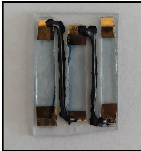
Figure 10: Picture of an unileg thermoelectric generator with only p-type legs made of PEDOT:Tos on glass
