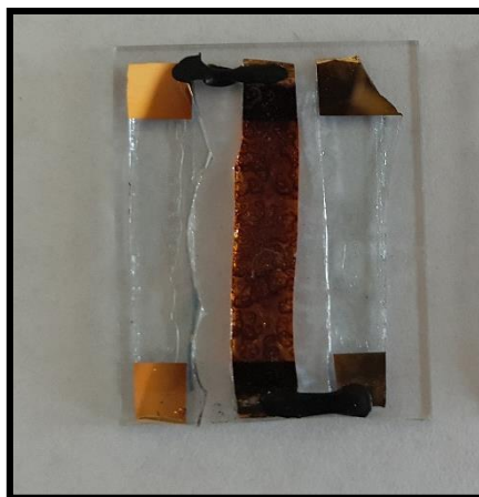
Figure 12: Picture of p-n-p three-legs thermoelectric generator with p-type legs made of PEDOT:Tos and n-type leg made with PCBM on glass
