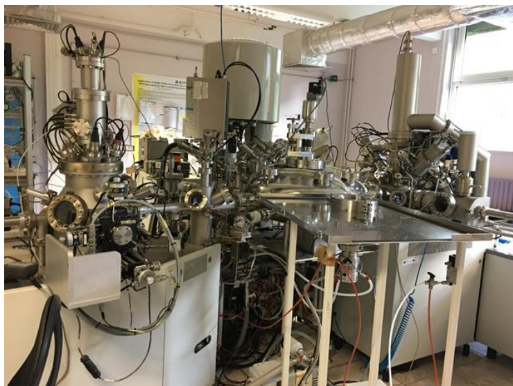
Figure 2.23 Surface analysis platform of Unité de Catalyse et Chimie du Solide (UCCS) located at Université de Lille 1. This platform encompasses a Kratos X-Ray Photoelectron Spectrometer (XPS-AXIS ULTRA DLD), a Low Ion Energy Ion Scattering (LEIS) instrument (Qtac 100) and a Time-of-Flight Ion Mass Spectroscopy (ToF SIMS5)
