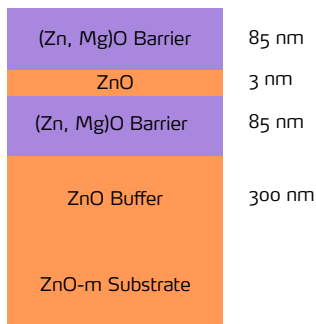
Figure 0.32.: Nominal samples' structures. The targeted value for the Mg content is 25 %.
