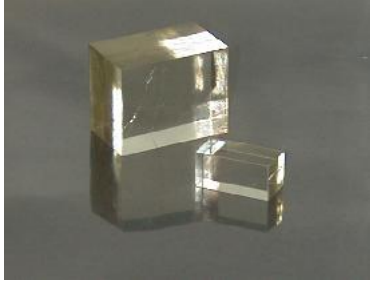
Figure 0.17.: Photo of a MgO single crystal (URL).
