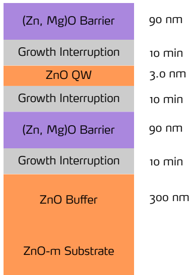
Figure 0.42.: Structure schematic of sample A. A growth interruption steps of 10 minutes was added between each epitaxial layer.
