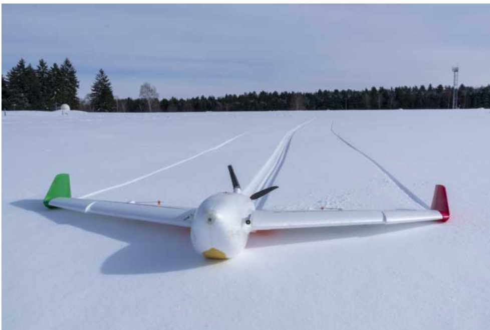
Figure 2-8: Drone equipped with Paparazzi on a mission for meteorological studies by MeteoFrance . Photo taken by Alexandre Bustico.
