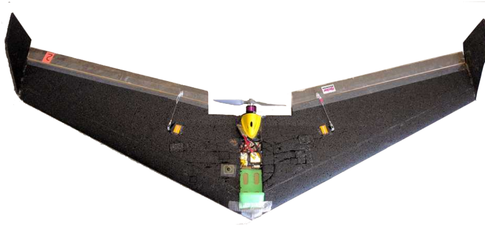
Figure 5-13: The flying-wing: ZAGI
