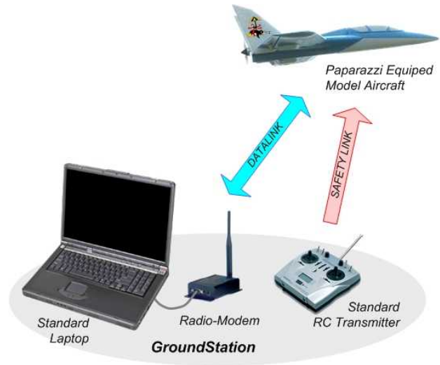
Fig. 1. Paparazzi autopilot system overview.
