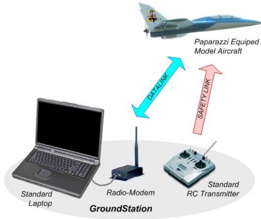
Figure 2-6: Paparazzi Autopilot System overview
