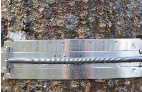
Appendix. 7: Dendrometers installed on the structural roots and the stem of walnut tree
