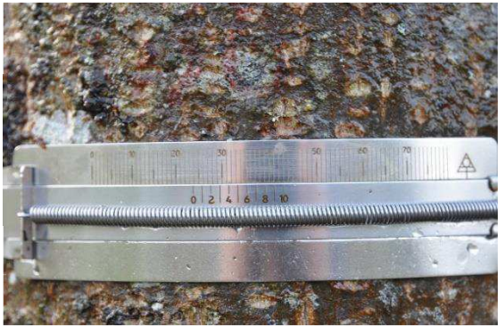
Appendix. 7: Dendrometers installed on the structural roots and the stem of walnut tree
