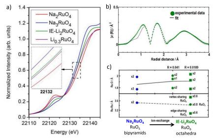
Figure II-44: a) Ru K-edge XANES spectra of  $Na_3RuO_4$ , IE- $Li_2RuO_4$ ,  $Na_2RuO_4$  and  $Li_{0.3}RuO_4$  (cf II.3.b.iv). b) Magnitude of the Fourier transforms of the  $k^2$ -weighted EXAFS oscillations of the IE- $Li_2RuO_4$  spectra with their fit, dot and plain lines, respectively. c) Ru-O and Ru-Ru distances and coordination numbers of  $Na_2RuO_4$  and IE- $Li_2RuO_4$  obtained from EXAFS analysis. Black solid and broken lines show average Ru-O and Ru-Ru distances, respectively.
