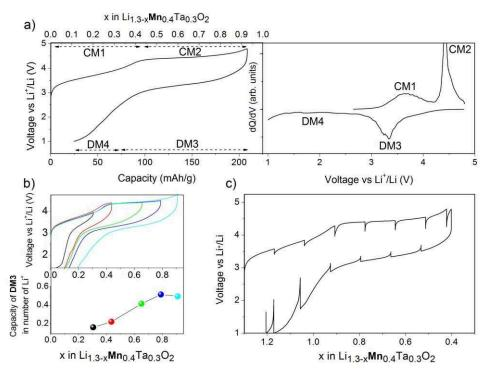
Figure III-14: a) Voltage-composition curve of the 1<sup>st</sup> galvanostatic cycle of LMTO, at C/20, together with its dQ/dV profile emphasizing the CM1, CM2, DM3 and DM4 processes. b) 1<sup>st</sup> galvanostatic cycle at different SOC together with the discharge capacity, in number of Li, of DM3 (>3 V) in the bottom panel. c) GITT of the 1<sup>st</sup> cycle of LMTO at C/20 with 5 hours rest every 3 hours.
