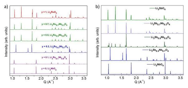
Figure II-5: Synchrotron X-ray diffraction patterns ( $\lambda = 0.414562 \text{ Å}$ ) for a) the Li<sub>3</sub>Ru<sub>y</sub>Nb<sub>1-y</sub>O<sub>4</sub> samples with y = 1, 0.7, 0.5, 0.3, 0.1 and 0 and b) the Li<sub>3</sub>Nb<sub>y</sub>Sb<sub>1-y</sub>O<sub>4</sub> samples with y = 1, 0.7, 0.5, 0.3, and 0.
