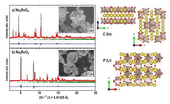
Figure II-36: Rietveld refinement of the SXRD patterns ( $\lambda = 0.41325 \text{ Å}$ ) for a) Na<sub>3</sub>RuO<sub>4</sub> and b) Na<sub>2</sub>RuO<sub>4</sub> together with SEM images. The structures of Na<sub>3</sub>RuO<sub>4</sub> and Na<sub>2</sub>RuO<sub>4</sub> are shown, top and bottom, respectively. Na, Ru and O are shown in yellow, gray and red, respectively.
