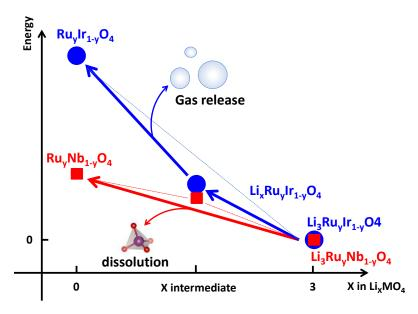
Figure II-35: Scheme explaining the impact of the stability of the  $MO_4$  end member with respect to the formation of intermediates and  $O_2$  gas release.
