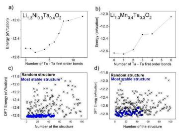
Figure III-23: a) and b) Variation of the average energy of the cation configuration, calculated by cluster expansion, with the number of first order Ta –Ta bonds for  $\text{Li}_{1.3}\text{Ni}_{0.3}\text{Ta}_{0.4}\text{O}_2$  and  $\text{Li}_{1.3}\text{Mn}_{0.4}\text{Ta}_{0.3}\text{O}_2$ , respectively.
