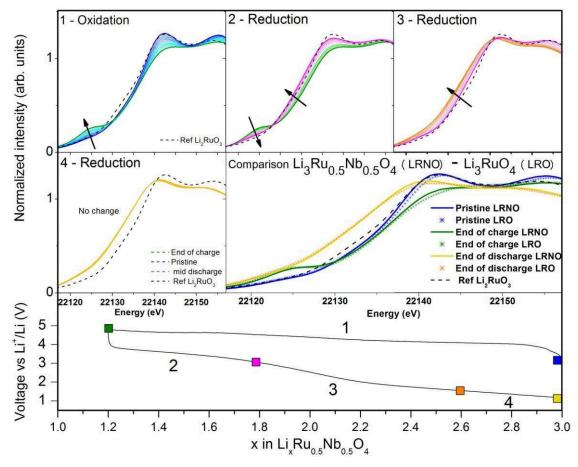
Figure II-30: Operando Ru K-edge XANES spectra for Li<sub>3</sub>Ru<sub>0.5</sub>Nb<sub>0.5</sub>O<sub>4</sub>. The XANES spectra for different regions of the galvanostatic curve are presented together with the electrochemical data, C/5, and a comparison of the spectra between Li<sub>3</sub>Ru<sub>0.5</sub>Nb<sub>0.5</sub>O<sub>4</sub> and Li<sub>3</sub>RuO<sub>4</sub>.
