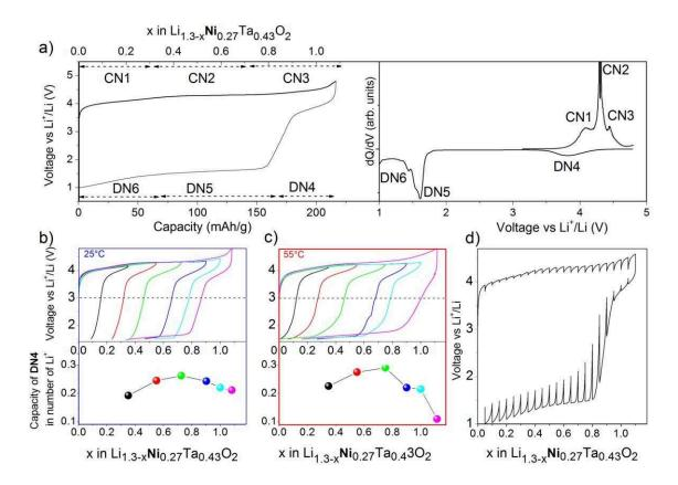
Figure III-3: a) Voltage-composition curve of the 1<sup>st</sup> galvanostatic cycle, C/20, and its dQ/dV profile, on the left and right panel respectively. b) and c) voltage-composition curve of the 1<sup>st</sup> cycle with different state-of-charge (top) together with the capacity of the DN4 (>3 V) depending on the SOC (bottom) at 25°C and 55°C. d) GITT measurement performed on the 1<sup>st</sup> cycle of LNTO at C/20 with 5 hours rest every hour.
