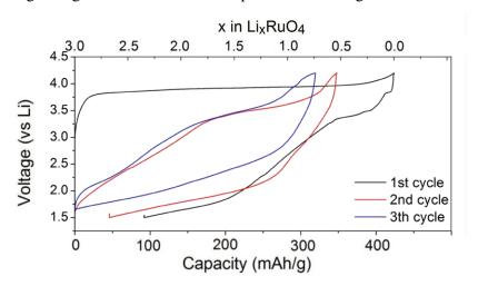
Figure II-18: 1st, 2nd and 3rd galvanostatic cycles for Li<sub>3</sub>RuO<sub>4</sub> at C/10 with 4.2 V – 1.5 V cutoff voltages
