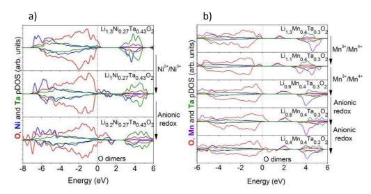
Figure III-25: a) and b) O, Ni, Mn and Ta pDOS in red, blue, purple and green, respectively for LNTO and LMTO at different state-of-charge.
