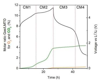
Figure III-20: OEMS results for LMTO, showing the evolution of the molar ratio between O2 and CO2 and the active material, in orange and green, together with the galvanostatic cycling data at C/30.
