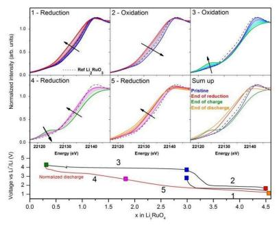
Figure II-24: Operando Ru K-edge XANES spectra for Li<sub>3</sub>RuO<sub>4</sub>. The XANES spectra for different regions of the galvanostatic curve, C/5, are presented together with the electrochemical data.
