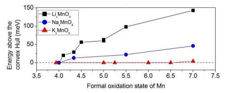
Figure II-47: Energy above the convex hull of the most stable structure depending on the oxidation state. Black, blue and red line stand for  $\text{Li}_x \text{MnO}_4$ ,  $\text{Na}_x \text{MnO}_4$  and  $\text{K}_x \text{MnO}_4$  systems, respectively.
