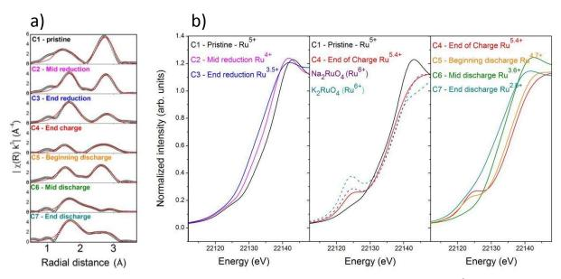
Figure II-26: a) Magnitude of the Fourier transforms (dotted line) and fit (plain line) of the  $k^3$ -weighted EXAFS oscillations of the MCR-ALS components. b) XANES spectra of the principal components obtained through MCR-ALS together with reference samples  $Na_2RuO_4$  and  $K_2RuO_4$  that have both  $Ru^{6+}$  oxidation state but in bipyramid ( $RuO_5$ ) and tetrahedral ( $RuO_4$ ) coordination, respectively.
