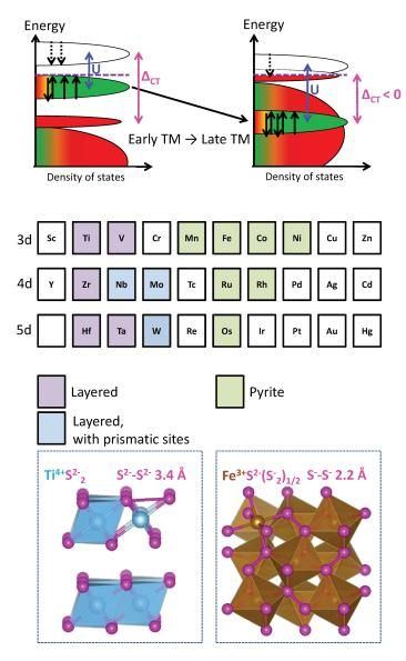
Figure I-8: Schematic presenting the evolution from a MH to a negative charge transfer regime in  $MS_2$  going from early to late transition metals (TM). This is exemplified by the structural transformation from a layered structure to a pyrite structure having S-S bonds of 3.4 and 2.2 Å, respectively.
