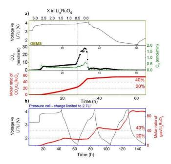
Figure II-23: OEMS measurements on  $\text{Li}_3\text{RuO}_4$  during galvanostatic cycling, C/10. a) Galvanostatic cycle, CO<sub>2</sub> and O<sub>2</sub> production rate, and integrated number of moles of CO<sub>2</sub> over the moles of active material are presented on the top, middle and bottom panel respectively. b) Pressure cell measurement limiting the charge before the massive gas release, e.g. at  $\text{Li}_{0.3}\text{RuO}_4$  composition.
