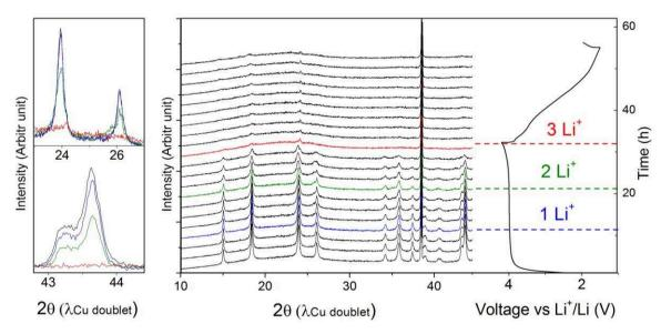
Figure II-19: In the middle panel are presented the XRD patterns collected during the charge and subsequent discharge of  $\text{Li}_3\text{RuO}_4$  operando. On the left side, specific patterns of the pristine, after the extraction of 1, 2 and 3 Li are shown in black, blue, green and red, respectively. On the right side the associated galvanostatic curve at C/10.
