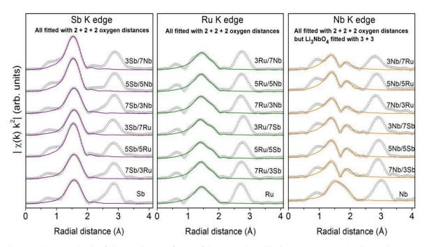
Figure II-10: Magnitude of the Fourier transforms of the EXAFS oscillations extracted at the Sb K-edge, Ru K-edge, and Nb K-edge for the left, middle and right panel respectively. The solid lines represent the model fitting for the M-O shell.
