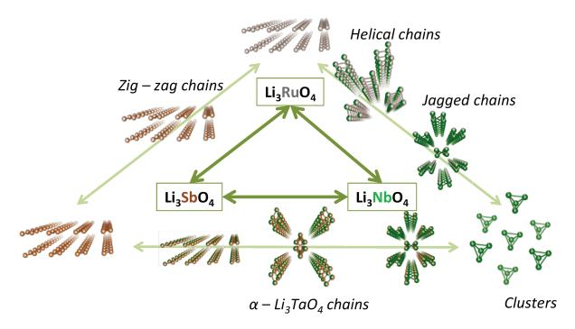
Figure II-6: Schematic of the structures of the  $\text{Li}_3\text{Ru}_y\text{Nb}_{1-y}\text{O}_4$ ,  $\text{Li}_3\text{Ru}_y\text{Sb}_{1-y}\text{O}_4$ , and  $\text{Li}_3\text{Sb}_y\text{Nb}_{1-y}\text{O}_4$  for y=1, 0.7, 0.5, 0.3, and 0. For each composition only the metallic framework, M-M bonds with M = Nb, Sb or Ru, are shown.
