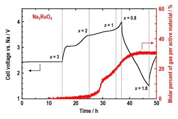
Figure II-41: Gas pressure measurement of the cell using pristine Na<sub>3</sub>RuO<sub>4</sub> operated at C/10. 15 hours OCV period was performed before starting charge. Black curve is a charge-discharge curve. Red curve is molar ratio gas per active material.
