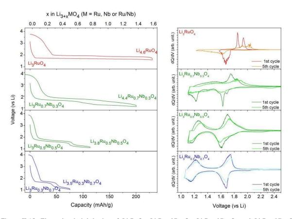
Figure II-15: Electrochemical behavior of  $Li_3RuO_4$ ,  $Li_3Ru_{0.7}Nb_{0.3}O_4$ ,  $Li_3Ru_{0.5}Nb_{0.5}O_4$  and  $Li_3Ru_{0.3}Nb_{0.7}O_4$  starting on discharge. (a) Voltage versus composition curves for the  $1^{st}$  cycle at C/10 with cutoff voltages of 1.40 V, 1.10 V, 1.05 V and 1.00 V b) Derivative dQ/dV curves for the  $1^{st}$  and  $5^{th}$  cycle.
