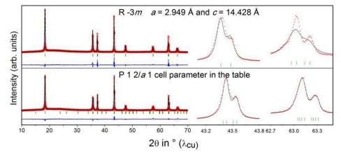
Figure II-3: Rietveld refinement of  $\text{Li}_3\text{Ru}_{0.5}\text{Ir}_{0.5}\text{O}_4$  using the structural model of  $\text{Li}_3\text{Ir}\text{O}_4$  described in R -3m (top) and the P 1 2/a 1 structural model of  $\text{Li}_3\text{Ru}\text{O}_4$  (bottom) together with zooms emphasizing the better fit using the structural model of  $\text{Li}_3\text{Ru}\text{O}_4$ .
