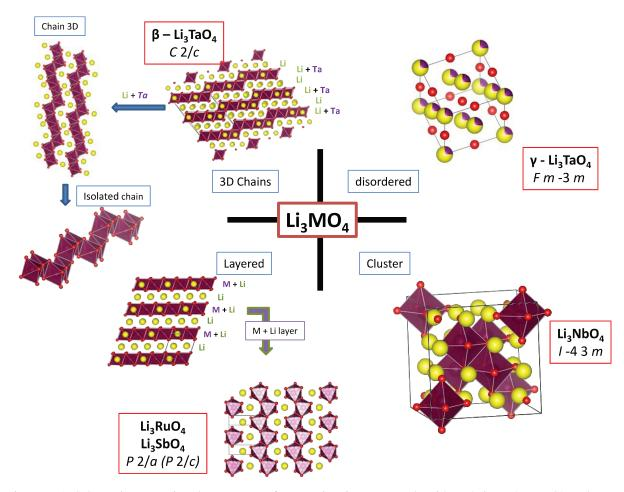
Figure II-1: Schematic presenting the structure of some Li<sub>3</sub>MO<sub>4</sub> compounds with M being Nb, Ru, Sb and Ta. All are rocksalt with different Li/M ordering.
