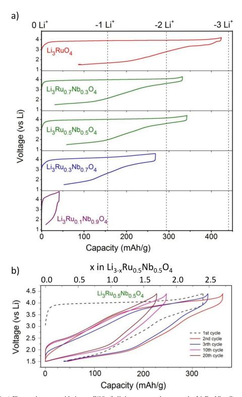
Figure II-29: a) First cycle upon oxidation at C/10 of all the compounds among the  $\text{Li}_3\text{Ru}_y\text{Nb}_{1-y}\text{O}_4$  series for y = 1, 0.7, 0.5, 0.3, 0.1 from the top to the bottom. b) Cycling performances for  $\text{Li}_3\text{Ru}_{0.5}\text{Nb}_{0.5}\text{O}_4$  cycled at C/10 with 4.4 V - 1.5 V cutoff voltages.
