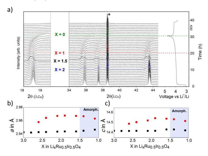
Figure II-33: Operando XRD for  $\text{Li}_3\text{Ru}_{0.5}\text{Ir}_{0.5}\text{O}_4$  during the 1<sup>st</sup> charge. a) show the XRD patterns in 18-19.5° and 34-44.5° range and the galvanostatic curve, C/10, from left to right. \* peak comes from the cell b) and c) present the evolution of the a and c cell parameter (fit in R-3m) during the charge obtained with Rietveld refinement for both phases.
