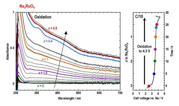
Figure II-40: Operando UV-visible spectra of Na<sub>3</sub>RuO<sub>4</sub> during the oxidation and the corresponding charge curve. Note that the charge doesn't show exactly the same profile as in a standard electrochemical cell. We attribute this difference to the absence of pressure applied on the electrode in the UV-visible cell. The UV-visible spectra were collected every one hour
