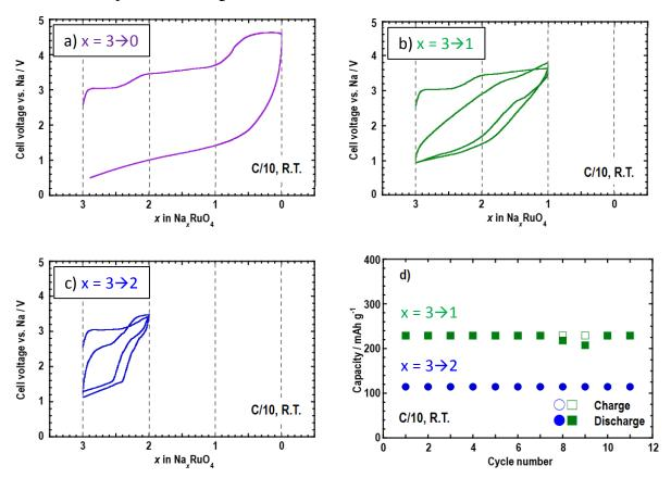
Figure II-37: The 1st and 2nd galvanostatic curves of Na cells with Na<sub>3</sub>RuO<sub>4</sub> cycled between a)  $x = 3 \rightarrow 0$ , b)  $3 \rightarrow 1$  and c)  $3 \rightarrow 2$ . d) Cycle performance of the cells with  $x = 3 \rightarrow 1$  (green square) and  $x = 3 \rightarrow 2$  (blue circle) in Na<sub>x</sub>RuO<sub>4</sub>.
