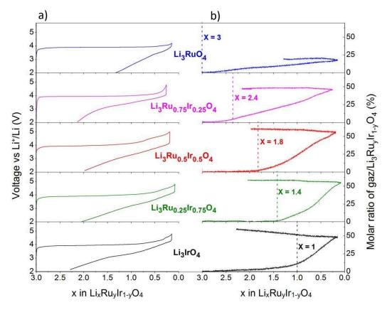
Figure II-32: a) 1st cycle of galvanostatic cycling, C/10, and b) molar ratio of the gas/active material evolution inside the cell for compounds among the solid solution  $\text{Li}_3\text{Ru}_y\text{Ir}_{1-y}\text{O}_4$  for y=1, 0.75, 0.5, 0.25 and 0 from top to bottom, at the left and right side, respectively. Dash lines indicate the gas pressure increase threshold.
