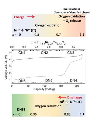
Figure III-13: Schematics presenting the charge compensation mechanism in  $Li_{1.3}Ni_{0.27}Ta_{0.43}O_2$ . The compensation during DN6 is marked as "DN6?" because still unclear.
