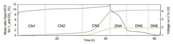
Figure III-10: Molar ratio of  $O_2/LNTO$  and  $CO_2/LNTO$  measured via mass spectrometry during galvanostatic cycling together with the voltage-composition curve, in orange, green and black, respectively. Note that the rate for the charge was C/40 and C/20 for the discharge.
