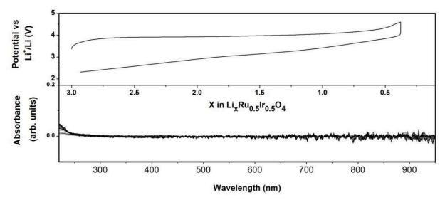
Figure II-31: Operando UV-visible spectroscopy for  $\text{Li}_3\text{Ru}_{0.5}\text{Ir}_{0.5}\text{O}_4$ . No sign of Ru dissolution is shown. Electrochemical cycle done at C/10.
