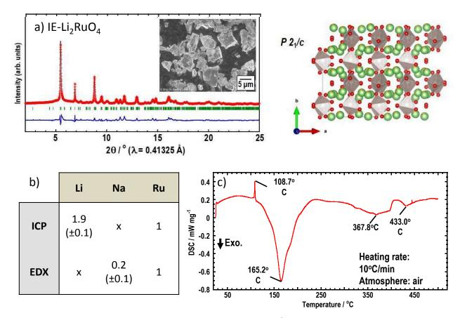
Figure II-43: a) Rietveld refinement of the SXRD pattern ( $\lambda$  = 0.41325 Å) with SEM image and structure of IE-Li<sub>2</sub>RuO<sub>4</sub>. b) Table showing the elemental analysis performed on IE-Li<sub>2</sub>RuO<sub>4</sub>. Traces of remaining Na were found by EDX. Note that Na quantification was not performed by ICP due to the utilization of NaOCl in the dissolution process. c) DSC of IE-Li<sub>2</sub>RuO<sub>4</sub> under air.
