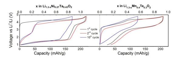
Figure III-2: shows the  $1^{st}$ ,  $2^{nd}$  and  $10^{th}$  cycles, at C/20, of  $Li_{1.3}Ni_{0.27}Ta_{0.43}O_2$  and  $Li_{1.3}Mn_{0.4}Ta_{0.3}O_2$ , respectively. x values for  $Li_xNi_{0.3}Ta_{0.4}O_2$  and  $Li_xMn_{0.4}Ta_{0.3}O_2$  are given for the  $1^{st}$  charge.
