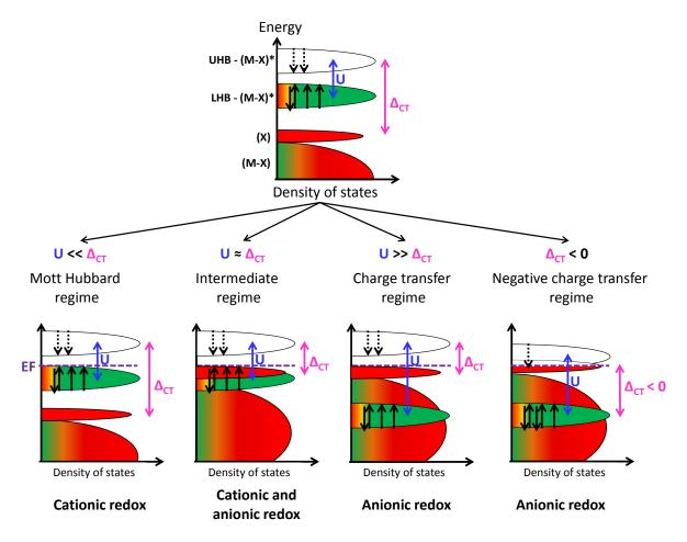
Figure I-7: Schematic presenting U and  $\Delta_{CT}$  together with the different electronic regimes that can be achieved depending on the relative value of U and  $\Delta_{CT}$ . UHB, LHB, (M-X)\*, (M-X), (X) and EF stand for Upper Hubbard band, Lower Hubbard band, M-X antibonding and bonding states, X lone pairs and EF Fermi level.
