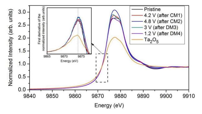
Figure III-17: Ex situ Ta L3-edge XANES spectra together with their first derivative curve for ex situ samples along the galvanostatic cycling of LMTO.
