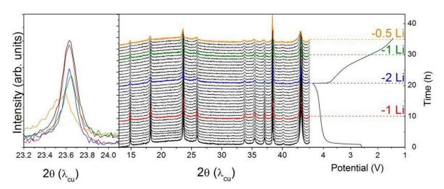
Figure II-28: In the middle panel are presented the XRD patterns collected during the charge and subsequent discharge of  $\text{Li}_3\text{Ru}_{0.5}\text{Nb}_{0.5}\text{O}_4$  Operando. On the left side, specific patterns of the pristine, after the extraction of 1, 2 Li and reinsertion of 1 Li and 0.5 Li are shown in black, red, blue, green and orange, respectively. On the right side the associated galvanostatic curve, C/10.
