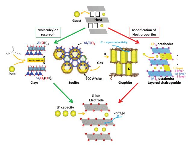
Figure I-2: Schematic of the general intercalation system (top) together with examples for ion storage systems such as clays and zeolites (middle left) and "property modification" systems, such as graphite and chalcogenides, (middle right). Li-ion electrodes combine both the properties as shown at the bottom.
