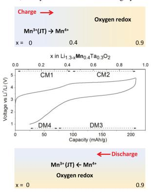
Figure III-22: Schematics representing the charge compensation mechanism for Li<sub>1.3</sub>Mn<sub>0.4</sub>Ta<sub>0.3</sub>O<sub>2</sub>
