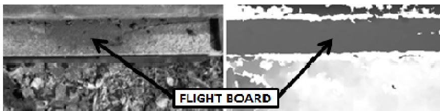
Fig. 1: Couple of intensity (left) / disparity (right) images provided by the stereo vision camera. The beehive is visible on the top. Bees take off/land on the flight board.
