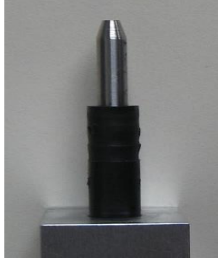
Figure 4-18: CO 2 jet setup scheme (left) [103] and picture of the exit nozzle (right).
