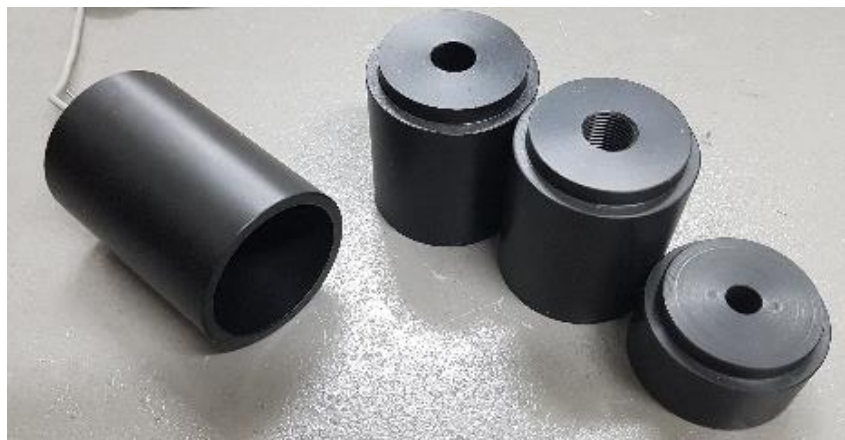
Figure 5-3: Atmospheric chamber for preliminary tests with different adaptive covers.
