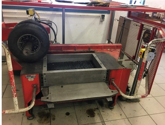
Figure 3.1 - French wheel compactor (NF EN 12697-33+A1:2007)
