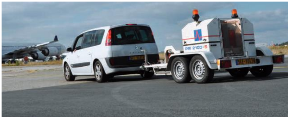
Figure 1.17 - Heavy Weight Deflectometer on a runway (STAC 2014)
