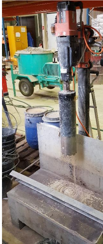
Figure 3.3 - Core drilling machine at the University of Lyon/ENTPE
