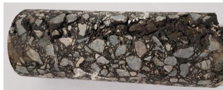
Figure 3.7 - Cylindrical sample of bituminous mixture cored too close to the surface and unfit for testing
