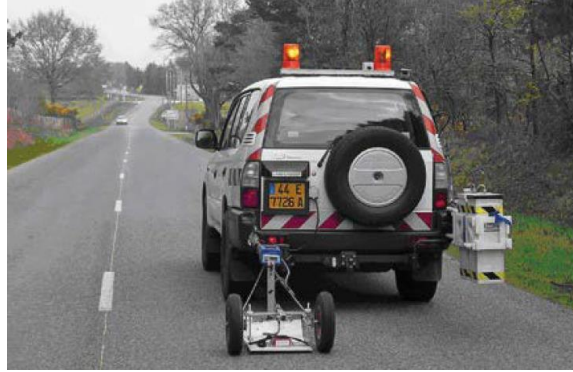
Figure 1.16 - Radar monitoring apparatus on a vehicle
