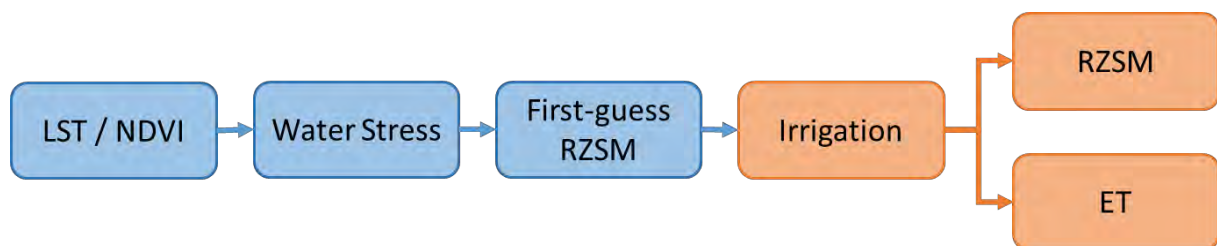
Fig. 3.2. Flowchart of the estimation of the main crop water budget components (irrigation, RZSM and ET) from the main intermediate variables.
