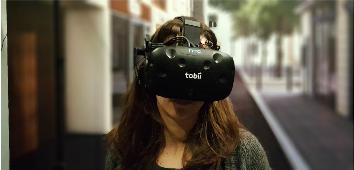
Figure 5.2 – Immersive virtual reality setup with position and orientation tracking combined with a Tobii eye-tracking device.
