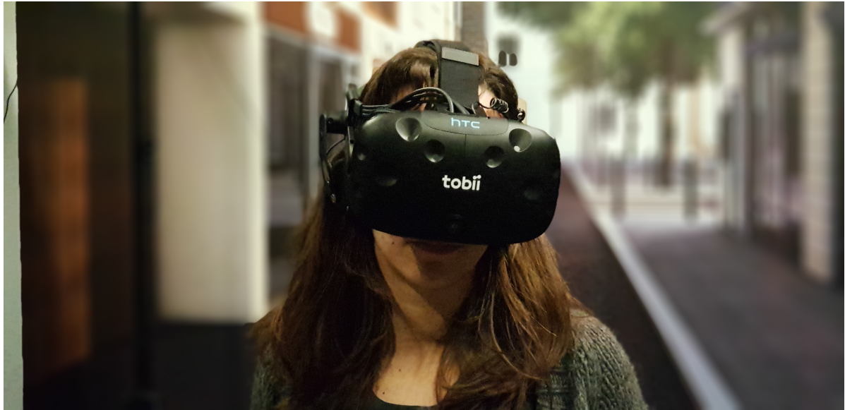
Figure 5.2 – Immersive virtual reality setup with position and orientation tracking combined with a Tobii eye-tracking device.
