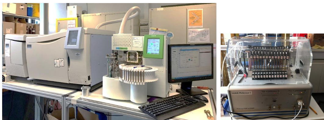
Figure II-1 The analytical TD-GC-MS system available at LaMP (left) and the automatic sampling module-SASS (Smart Automatic Sampling System) installed at the puy de Dôme station (right).
