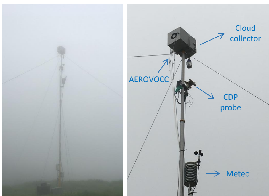
Figure III-6 Presentation of the instruments deployed during the BIOMAIDO field campaign in 2019 for collecting gaseous compounds and cloud droplets.
