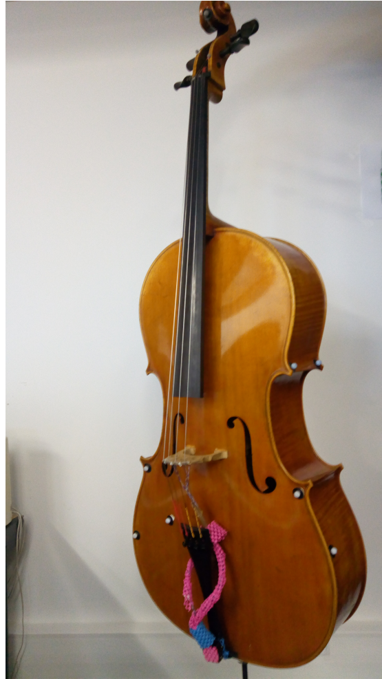
FIGURE 4.16: Here we see four markers on the front, three markers on the side, three markers on the scroll, two temporary markers on the nut, and three temporary markers on the bridge.
