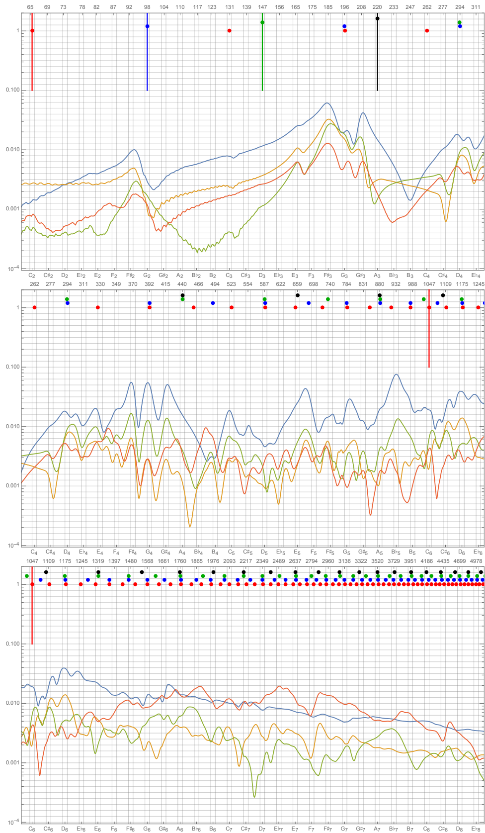
FIGURE 2.10: Mobility measurements (in \frac{m}{N \cdot s} ) of Cello B. Horizontal force, horizontal motion (blue); horizontal force, vertical motion (yellow); vertical force, horizontal motion (green); vertical force, vertical motion (red).
