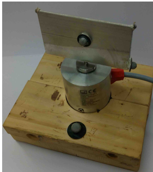
FIGURE 3.6: An HBM U1A force transducer with an aluminum blade measures bow forces up to 10 N for calibrating the hair compliance model.
