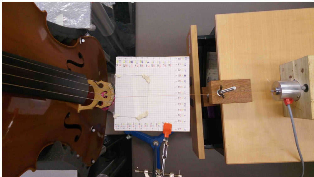
FIGURE 4.4: A HBM U1A force transducer is used to measure the magnitude force applied to the string when the wire breaks. Sliding the force transducer along the surface of the table ensures the force is applied within the bridge plane. A guide post is used as a reference to set the angle of the applied force.
