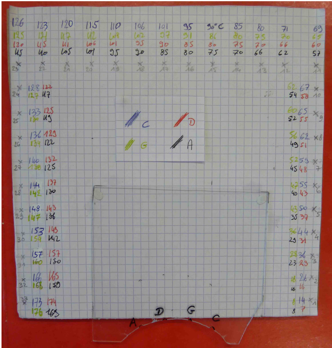
FIGURE 4.5: A protractor along with a guide post is used to set the angle of the applied force relative to a global reference frame. The protractor registers against the strings and curve of the bridge. The gridded paper indicates the two reference axes in the plane of the bridge. Several positions are marked along the edge of the protractor. Four angles are marked at each position corresponding to the angles of the lines connecting the point to each of the four strings.
