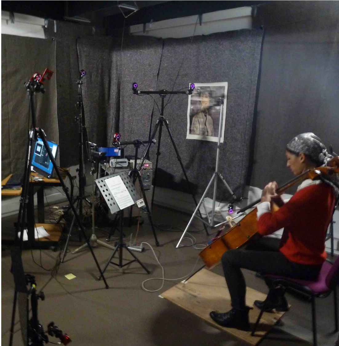
FIGURE 4.9: Here we can see the positions of eight of the ten motion capture cameras. The two cameras mounted near the ceiling are out of frame.
