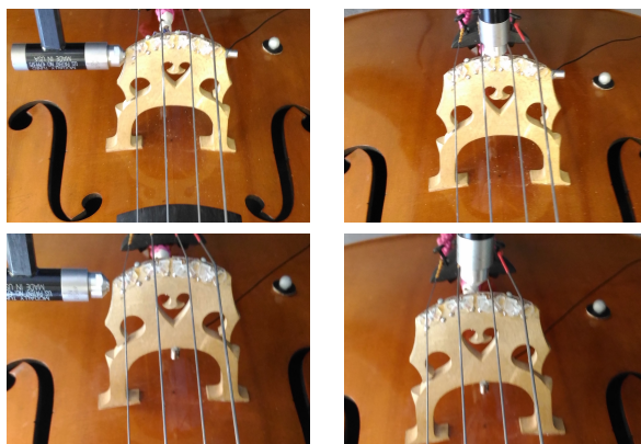
FIGURE 2.7: Bridge mobility and radiation transfer function measurements conducted with horizontal forces (left figures) and vertical forces (right figures). The horizontal acceleration is measured with the accelerometer on the side of the bridge (top figures) while the vertical acceleration is measured with the accelerometer between the legs (bottom figures). The microphone was located 160 cm in front of the cello.
