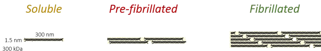
Figure V-2 : Three states of collagen : soluble triple helices (acidic media), pre-fibrillated state to create small building blocks (pH 4 ) and fibrillated collagen (pH ca. 7).
