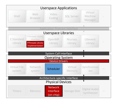
Figure 1.7 – Subutai components are highlighted in red in the computing stack. Subutai only requires changes in the (i) on-chip NI, (ii) OS NI driver and (iii) PThreads implementation. Additionally, a new scheduling policy (in blue) is explored in this work as an optional optimization.
