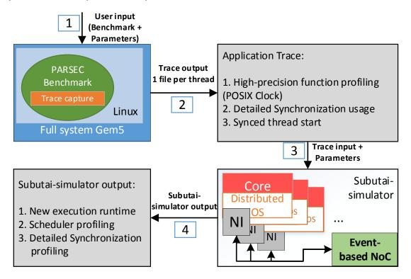
Figure 6.1 – Experimental setup for Subutai evaluation.
