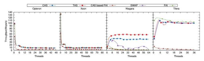
Figure 2.2 – Throughput of different atomic operations on a single memory position [DGT13].
