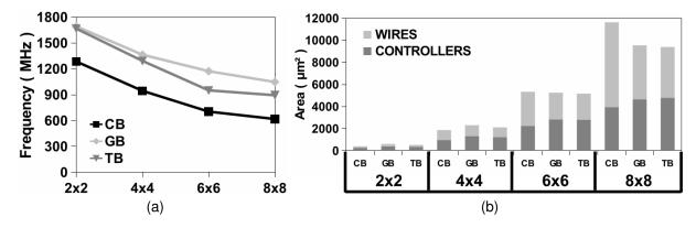
Figure 3.12 – (a) Optimal frequencies and (b) area overhead running at 600MHz for all analyzed topologies [AFA<sup>+</sup>12].
