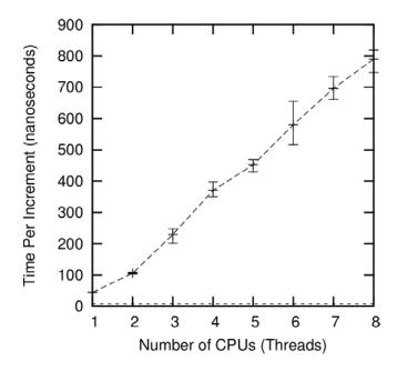
Figure 2.1 – Atomic increment scalability on a Nehalem Intel processor [McK19a].
