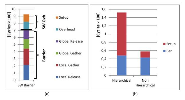
Figure 3.13 – The barrier cost of (a) SW and (b) HW implementation in cycles [AFA+12].
