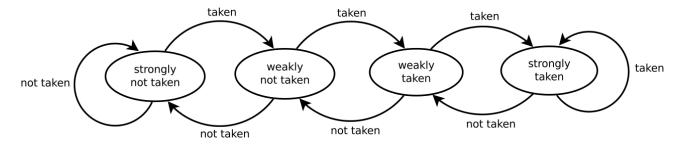
Figure 4.8 – 2-bit saturating counter for branch prediction [Dia19].
