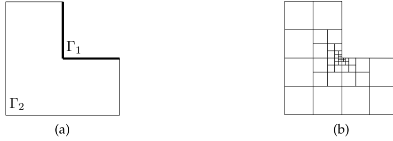
Figure 4.3 – Left: Fichera corner domain. \Gamma_1 corresponds to the thicker boundary part, \Gamma_2 to the rest of the boundary. Right: computational mesh.
