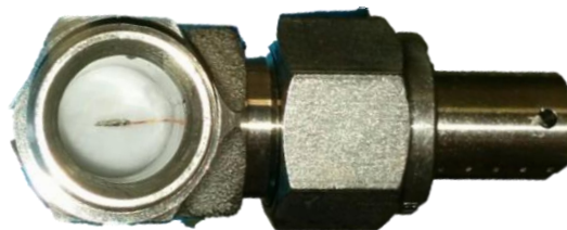
Figure A1.3 | Photograph of the Li metal reference electrode at the tip of an enamelled copper wire placed inside the three-electrode Swagelok cell.
