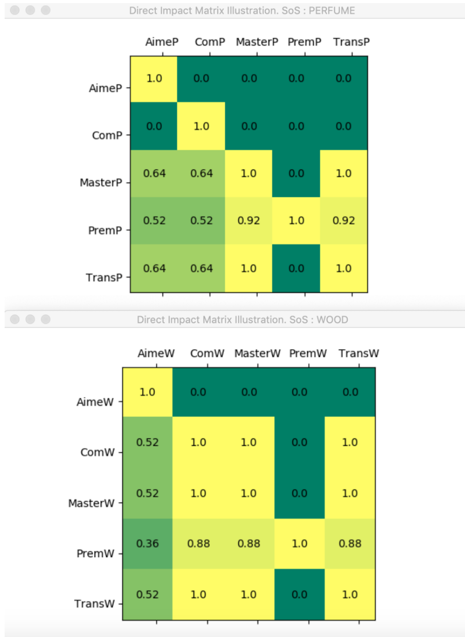
Figure 5.20: Direct impacts calculations by CS. Calculations of PERFUME SoS are at the top. Calculations of WOOD SoS are at the bottom.
