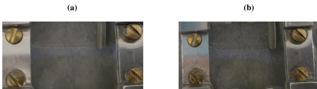
Figure 4.4 Photos of hydrogels (a) maintained under specified deformation at 60 °C (b) unloaded (i.e., at zero external force) at 60°C
