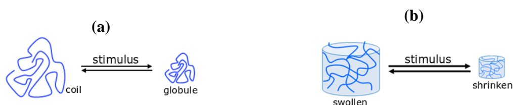
Figure 1.18. Schematic representation of polymer phase-separation induced by a stimulus for (a) a polymer chain exhibiting a coil-globule transition and (b) a hydrogel
